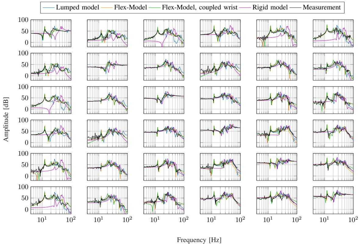
Fig. 5: Matrix of FRFs from motor torque (columns) to motor acceleration (rows) for one robot pose.
