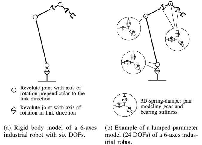
Fig. 2: Rigid multibody model and example of a lumped parameter model of a 6-axes industrial robot.
