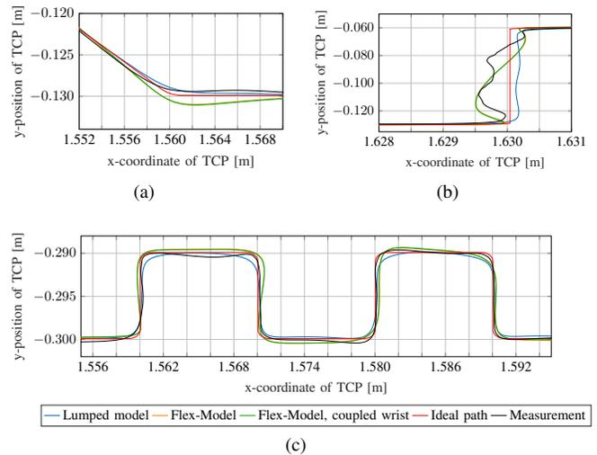
Fig. 7: Enlarged sections of the test path; simulated and measured TCP positions with an experimental path controller.
