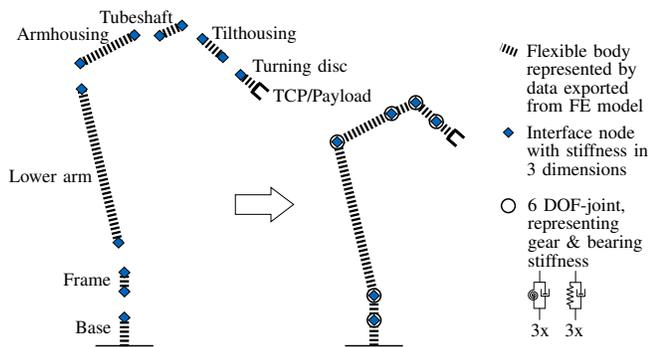
Fig. 3: Schematic drawing of the S-node Flex-Model.
