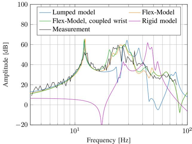
Fig. 6: FRF from motor torque of axis 3 to acceleration of motor 1 for one robot pose.
