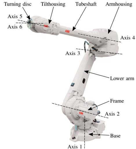
Fig. 1: 6-axes industrial robot.
