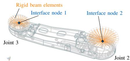
Fig. 4: Interface nodes of the lower arm.
