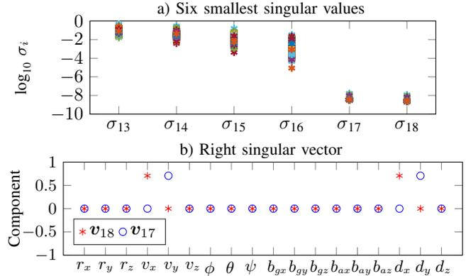
Fig. 5. SVD of the observability matrix for the full state model: a) six smallest singular values in logarithmic scale at different time instants, b) right singular vector  $v_{17}$  and  $v_{18}$  of the second smallest and smallest singular value, respectively.
