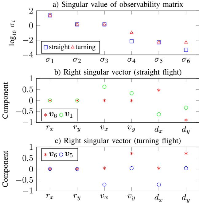
Fig. 4. SVD of the observability matrix for the 2D model: a) singular values in logarithmic scale in a straight and a turning flight, b) right singular vector  $v_6$  and  $v_1$  of the smallest and largest singular value in the straight flight, respectively, c) right singular vector  $v_5$  and  $v_6$  of the two smallest singular values in the turning flight, respectively.
