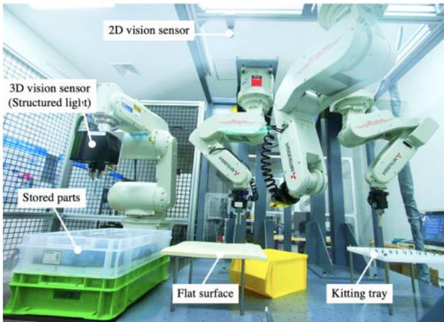
Fig. 6. Experimental system. The system is made of four 6-DoF industrial arms made by Mitsubishi Electric Corporation, one structured light based 3D vision sensor for bin-picking, and one 2D vision sensor for recognizing the pose of an isolated part.
