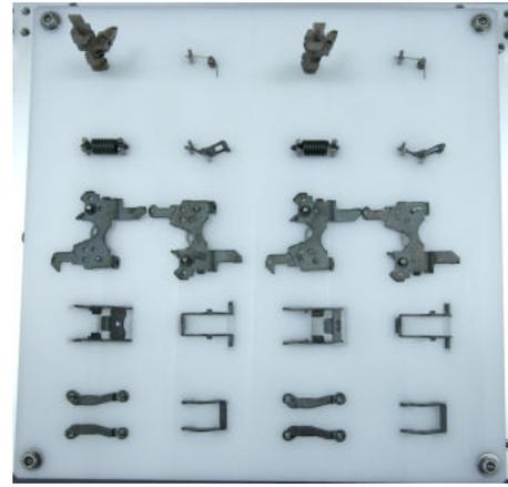
Fig. 7. Aligned parts by the proposed system in the kitting tray.
