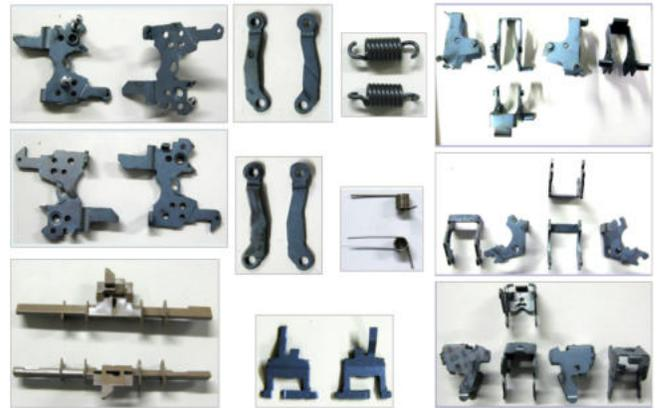
Fig. 8. Eleven types of target parts. These parts are used to assemble an industrial breaker. The parts sizes range from about 5 millimeters to 40 millimeters. The shapes are various, including plain, cylindrical, box, and more complicated types.
