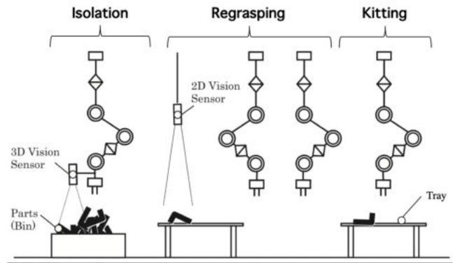
Fig. 2. Overview of the proposed robotic parts feeder.
