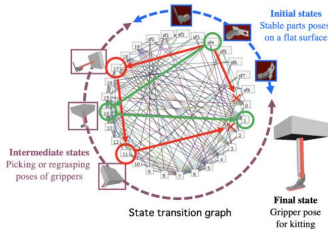
Fig. 4. Connecting the grasp configurations into a graph for regrasp planning. Each grasping configuration (identified by a pose) is treated as a node. Two nodes are connected if they share a common grasp configuration.
