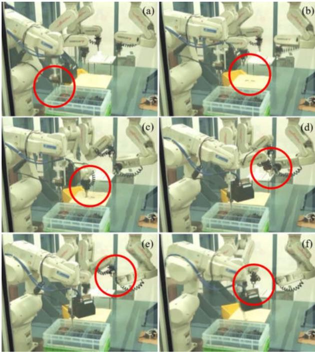
Fig. 9. Sequence of snapshots showing the real-world executions. (a) The first robot isolates some parts. (b) Pose estimation using the 2D vision sensor. (c)-(e) Regrasping. (f) Kitting. For more details, please watch the attached video.
