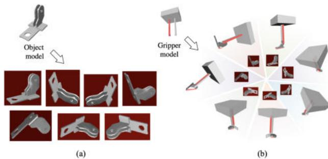
Fig. 3. State definition for regrasp planning – I. (a) Stable poses on a flat surface. (b) Accessible grasp configurations associated with the stable poses.
