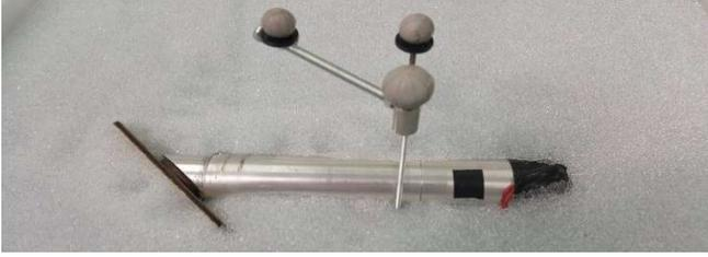
Figure 9 - Reflective markers connected above the robot so that trajectory can be measured while the robot is underground.
