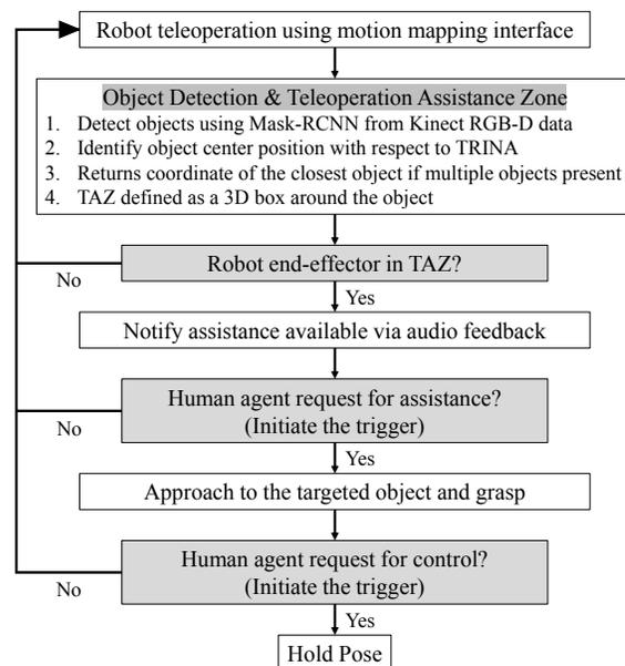
Fig. 3: Autonomous Grasping Function for Teleoperation Assistance.
