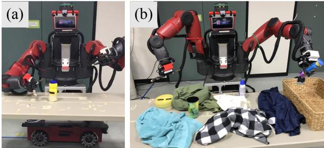
Fig. 5: Teleoperation tasks: (a) reaching-to-grasp an individual object; (b) collecting multiple objects in a cluttered counter workspace.
