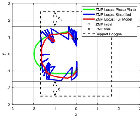
Fig. 3: ZMP loci of constrained motion planning vs. phase plane method.
