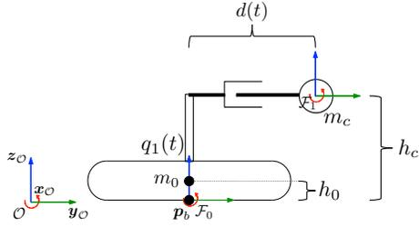
Fig. 2: Schematic diagram of a simplified feller buncher.
