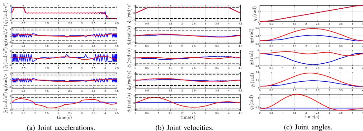
Fig. 4: Joint accelerations (a), velocities (b), and angle (c) plots. Blue line indicates results from the simplified model, red line indicates results from the full model, and black dashed lines indicate constraints. Note that all of the values related to  $q_5$  are zero due to this DoF being reduced in the simplified model.
