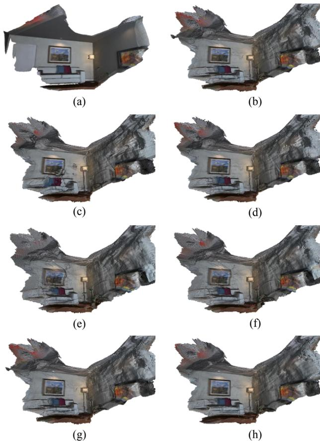
Fig. 4. **3D reconstruction results on ICL-NUIM dataset.** (*kt0* sequence). 3D meshes are extracted from the global TSDF according to the following weight options: (a) ground truth (b) constant (c) linear (d) exponential (e) min-depth based (f) minmax-depth (g) truncated uncertainty (h) normalized uncertainty
