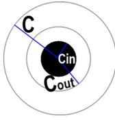
Fig. 1. Scheme showing distance in which the collision avoidance is activated ( $c_{out}$ ), the considered robot size for the collision avoidance ( $c_{in}$ ) and the communication range of a robot ( $c$ ).
