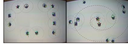
Fig. 4. Experiment with 11 robots divided in 6 groups,  $N_k = \{2, 1, 3, 2, 2, 1\}$ ,  $k \in \{1, \dots, 6\}$ . Circles are the communication radius  $c$ .
