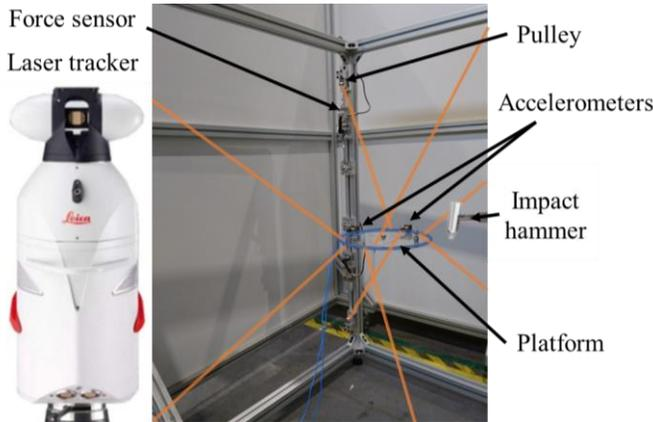
Figure 9. Experimental setup.
