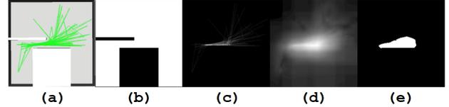
Fig. 3. (a) An example training environment overlain with motion traces. (b) Model input obtained post raster scan. (c) Motion trace image based on  $\mu$ -criticality of each pixel. (d) Saliency map obtained from the motion trace image. (e) Label obtained after binning the saliency map based on pixel intensity.
