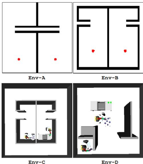
Fig. 5. Env-A and Env-B are the  $SE(2)$  environments used to evaluate the model. Red dots represent the start and goal configurations. Env-C and Env-D are the 10-DOF test environments used to evaluate the model. The robot is placed at the start and goal configurations. Test environments are unseen to the network (they were not used in the training set of problems).
