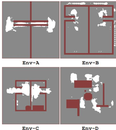
Fig. 6. Network output for the test environments shown in Figure 5. The  $\mu$ -criticality of the output is as follows:  $\mu(\text{Env-A}) = 0.604$ ,  $\mu(\text{Env-B}) = 1.351$ ,  $\mu(\text{Env-C}) = 0.538$ , and  $\mu(\text{Env-D}) = 0.398$ .
