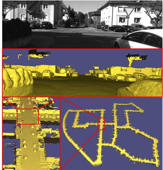
Fig. 1: Reconstruction of KITTI odometry sequence 00 with a closer look at an intersection that was passed multiple times during recording.
