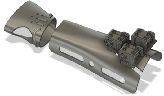
Fig. 3: CAD model of exoskeleton supports on the hand and on the forearm.
