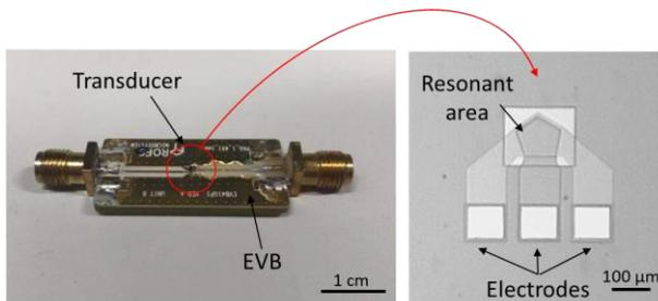
Figure 2. Picture of the microparticle manipulation system. Enlarged view is the microscope image of the gigahertz transducer with a pentagonal resonant area.
