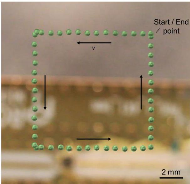
Figure 8. Control of the in-plane position of a microparticle following a square trajectory. The overlapped image shows the moving trajectory of the particle, and the arrows indicate the moving direction. The translational velocity is 0.4 mm/s.
