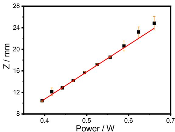
Figure 6. Relationship between the trapping height of the microparticle and the applied electric power. Error bars represent standard deviations.
