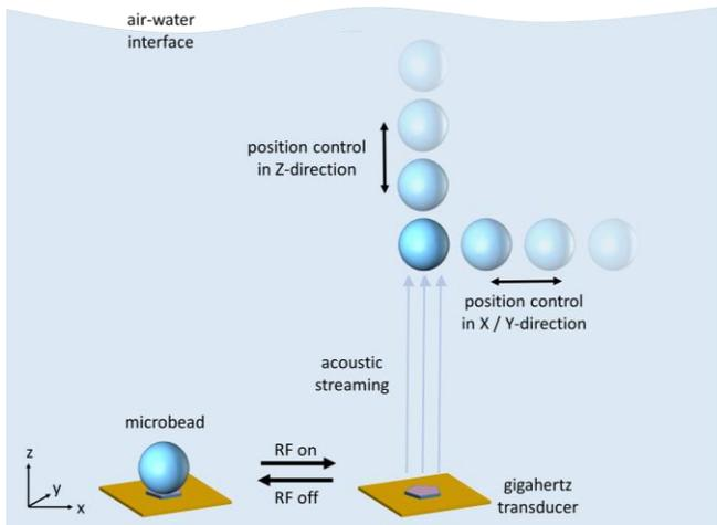
Figure 1. Schematic of the acoustofluidic tweezers for the microparticle manipulation. The stable 3D trap is generated in water with the acoustic streaming induced by the gigahertz ultrasonic transducer.
