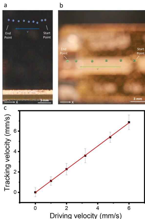
Figure 7. Control of the horizontal position of the microparticle by moving the fluidic tweezer. (a) Overlapped image of the side view of moving a particle at  $\sim 0.1$  mm/s; (b) Overlapped image of the top view of moving a particle at  $\sim 0.3$  mm/s. Arrows show the translational direction of the particle. (c) Tracking velocity of the particle versus the driving velocity of the motorized stage. Error bars represent standard deviations.
