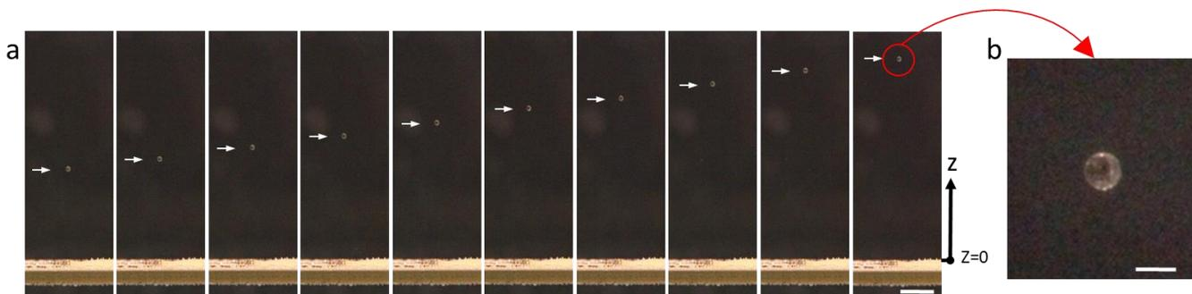
Figure 5. Control of the particle position in the Z direction by tuning the applied power. (a) From left to right: input power increases from 0.4 W (25.95dbm) to 0.7 W (28.45 dBm) with a step of 0.25 dB. White arrows indicate the position of the particle in each frame. Scale bar is 4 mm. (b) Enlarged view of the trapped glass microparticle. Scale bar is 500 $\mu$ m.
