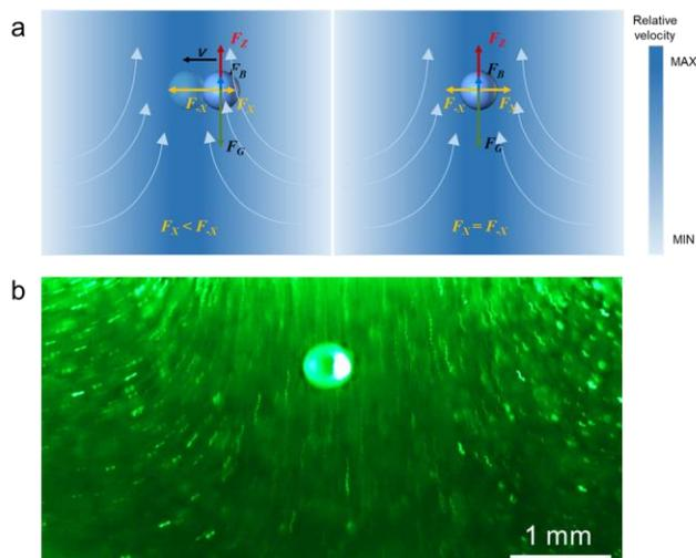
Figure 4. (a) Force diagram of the microparticle at different horizontal positions. Light-blue arrows indicate the fluid flow direction. Fluid velocity variation along X-axis is illustrated by background color variation. The off-center particle (as shown in the left picture) experiences a net horizontal force pointing towards the center where the forces balance (as shown in the right picture). (b) Recorded streamlines around the levitated particle.
