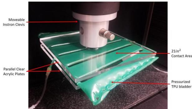
Figure 5. Test setup to determine the pressure the bladder imparts on user.
