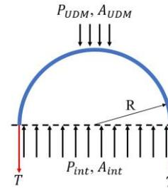
Figure 7. Free body diagram of the cross-section of the human forearm sized bladder used to determine the pressure the UDM imparts on user.  $L$  is the length of the walls of the bladder in and out of the page.  $P_{int}$  and  $A_{int}$  represent the internal pressure and cross-sectional area respectively. Likewise,  $P_{UDM}$  and  $A_{UDM}$  represent the pressure and contact area imparted on the bladder by the UDM.
