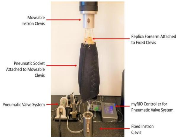
Figure 8. Test setup for axial loading tests.
