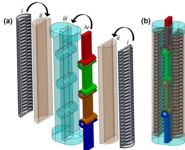
Figure 4. (a) Components of the manipulator: *i*) inextensible nylon fiber as a reinforcement element, *ii*) unreinforced silicone actuator, *iii*) encapsulation layer, *iv*) SCS. (b) completed manipulator.
