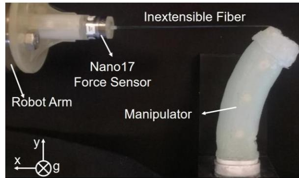
Figure 10. Experimental setup for manipulator stiffness measurement.
