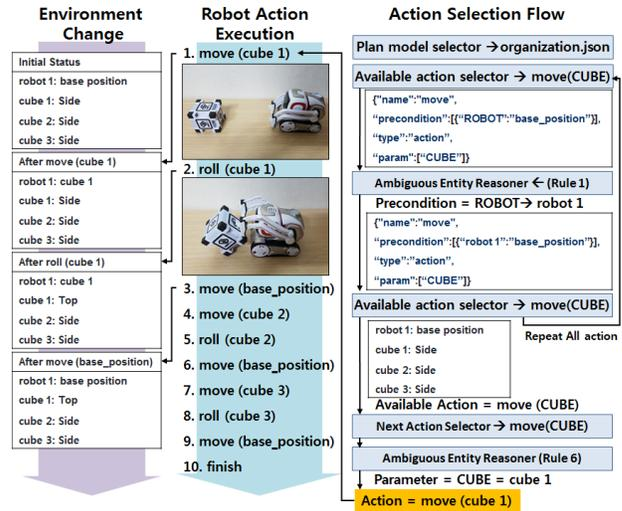
Figure 4. Action execution based on generated plan model
