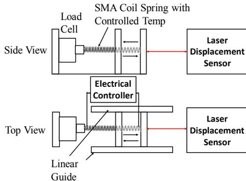
Fig. 1: Experimental Setup for measuring force-displacement relationship of the SMA coil spring.
