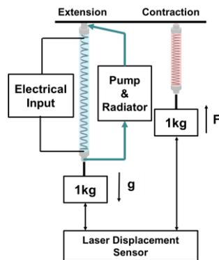
Fig. 7: Experimental setup for measuring actuation times of muscle-like SMA actuator with coolant vascular.
