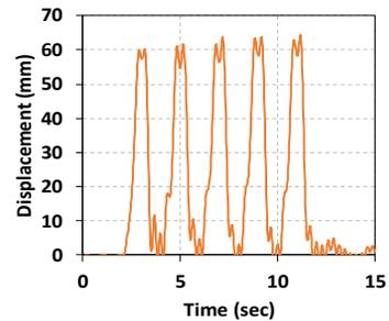
Fig. 9: Cyclic actuation performance of muscle-like SMA actuator with coolant vascular.
