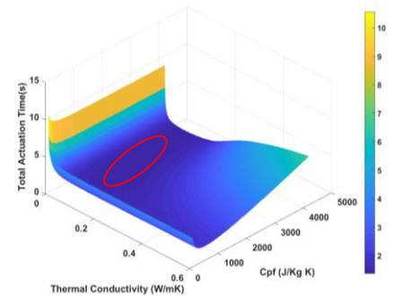
Fig. 5: Simulation results of actuation time of the muscle-like SMA actuator with coolant vascular.
