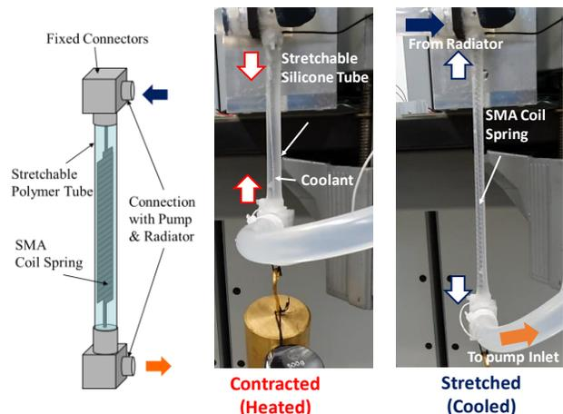
Fig. 3: Muscle-like SMA actuator with coolant vascular.
