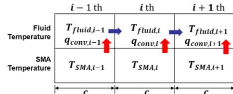
Fig. 4: Temperature profiles and heat transfer of Muscle-like SMA actuator with coolant vascular by segments.
