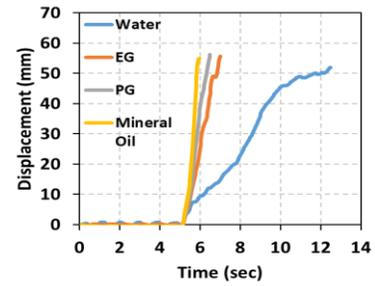
Fig. 8: Experimental results of contraction time of muscle-like SMA actuator with coolant vascular.
