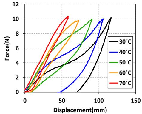
Fig. 2: Force-displacement relationship of the SMA coil spring.
