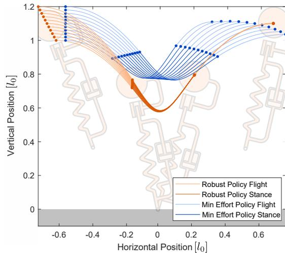
Fig. 5. Simulation results of the open loop plans for the robust policy and the minimum effort policy. The robust policy (orange) has an apex height error of less than  $0.001 [l_0]$  and an apex velocity error of less than  $0.001 [\sqrt{gl_0}]$  for all disturbance cases. The swing leg of the robust policy is a product of the optimization while the minimum effort policy uses ground speed matching.
