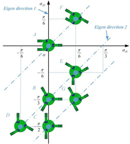
Fig. 8 Eigen directions and some postures of the abduction-adduction joints described in actuator space.
