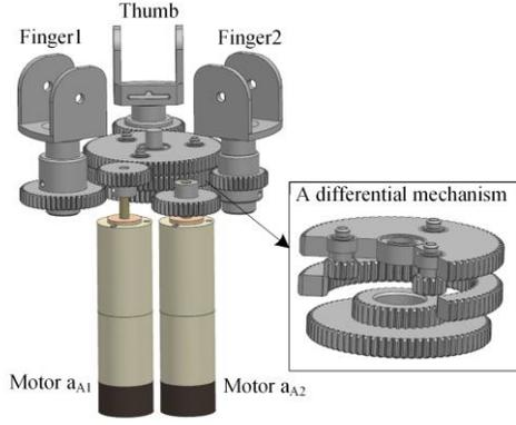
Fig. 7 A gear differential mechanism for 2-DOFs abduction-adduction movements of three digits.
