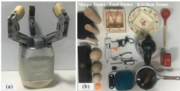
Fig. 10 (a) a synergy-driven three-fingered hand. (b) Objects selected for experiments.
