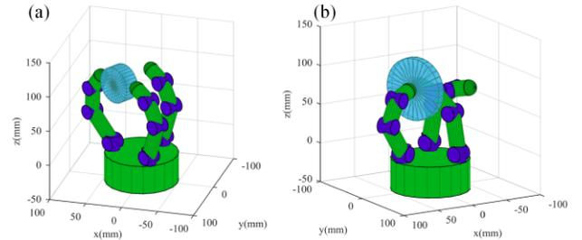
Fig. 9 Two typical grasping postures. (a) Fingertip grasping between the thumb and a finger (corresponds to Posture F in Fig. 8), (b) lateral pinch (corresponds to Posture G in Fig. 8).
