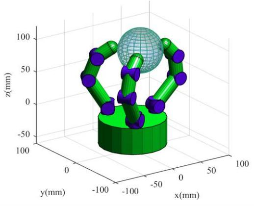
Fig. 2 Joint arrangement of the robot hand.
