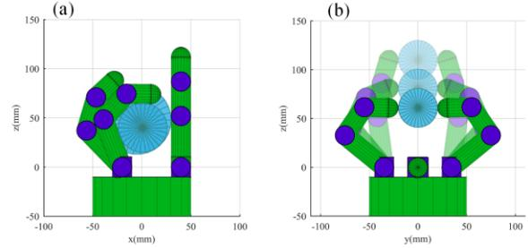
Fig. 6 The two fingers (a) adapt to a multi-diameter shaft, and (b) grasp a sphere of different positions
