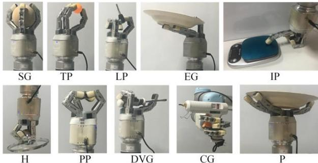
Fig. 11 Grasping demonstration with the prototype. Eight grasping types: H: hook; SG: spherical grip; TP: tripod pinch; EG: extension grip; DVG: diagonal volar grip; LP: lateral pinch; PP: pulp pinch; CG: cylindrical grip. Two non-grasping postures: IP: index pointing/pressing; P: platform.
