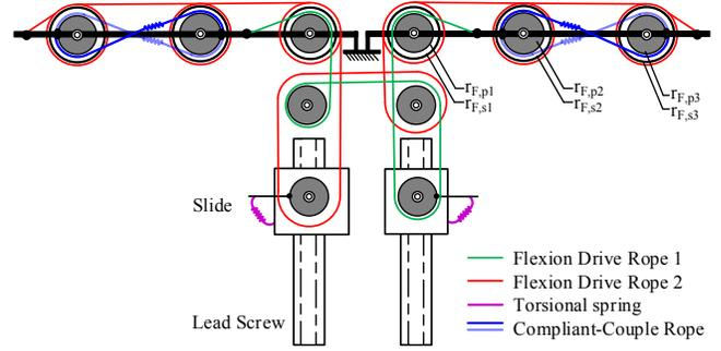
Fig. 5 The transmission for flexion-extension of the two fingers. Note that the extension drive rope 1 and 2, opposite to the corresponding flexion drive rope, are not appeared.
