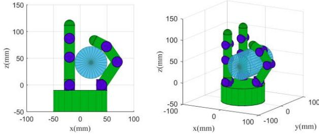
Fig. 4 The thumb adapts to a cylinder.
