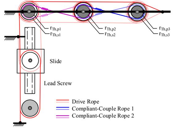
Fig. 3 The transmission for flexion-extension of the thumb.
