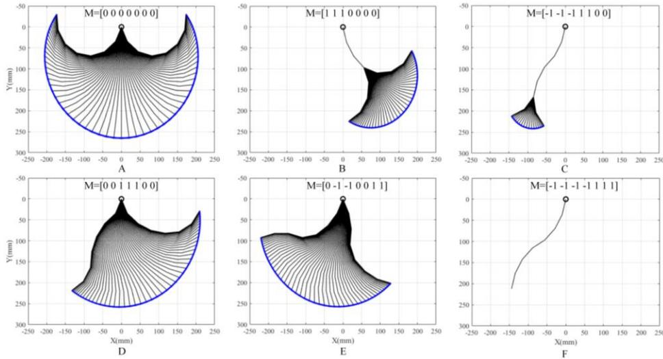
Fig. 4. One example for each type of configuration of cable-driven articulated soft robot. (A) Free bending. (B) Start one-side locking. (C) Start two-side locking. (D) Non-start one-side locking. (E) Non-start two-side locking. (F) Full locking.
