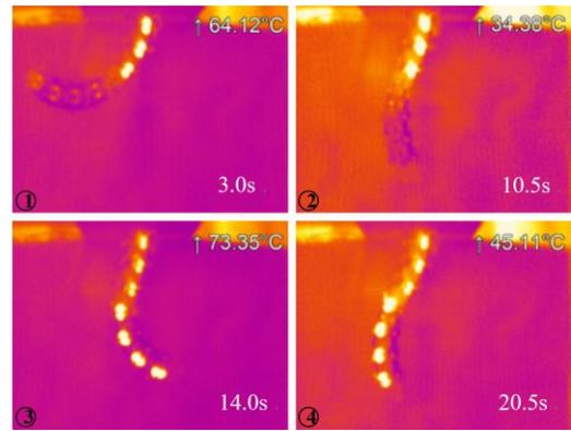
Fig. 8. Thermal view of the locking process of the robot arm. ① → ② shows right locking mode of joint 1-joint 3, and ③ → ④ shows left locking mode of joint 4-joint 7.
