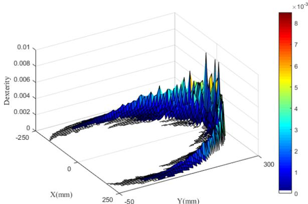
Fig. 6. Dexterity distribution in workspace. The color indicates the dexterity at each position patch.
