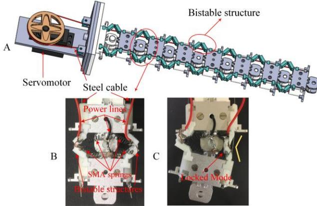
Fig. 2. (A) 3D model illustration of the articulated soft robot arm. (B) A prototype of the joint. (C) The joint is locked.
