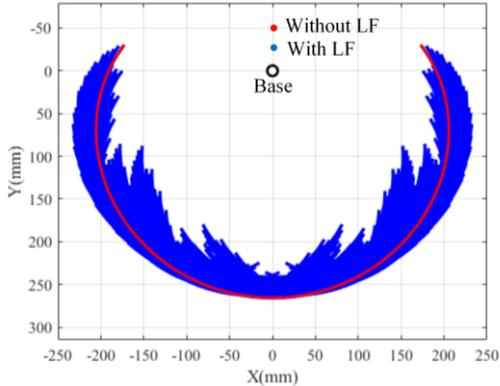
Fig. 5. Comparison of workspace between robot arm with locking function (blue area) and that without locking function (red curve). The resolution for this workspace is 500×500.
