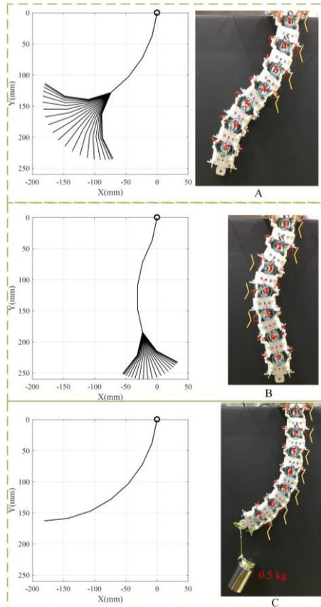
Fig. 7. The demonstration of articulated soft robot arm. (A) Right locking: joint 1 to joint 4, free bending: joint 5 to joint 7. (B) Right locking: joint 1 and joint 2; left locking: joint 3, joint 4, and joint 5; free bending: joint 6 and joint 7. (C) Full locking on the right side.
