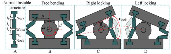
Fig. 1. Example of bistable structures in an articulated joint.
