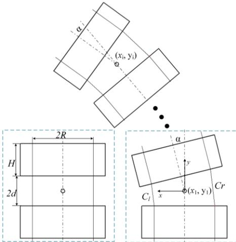
Fig. 3. brief sketch of the joint cable-driven motion.
