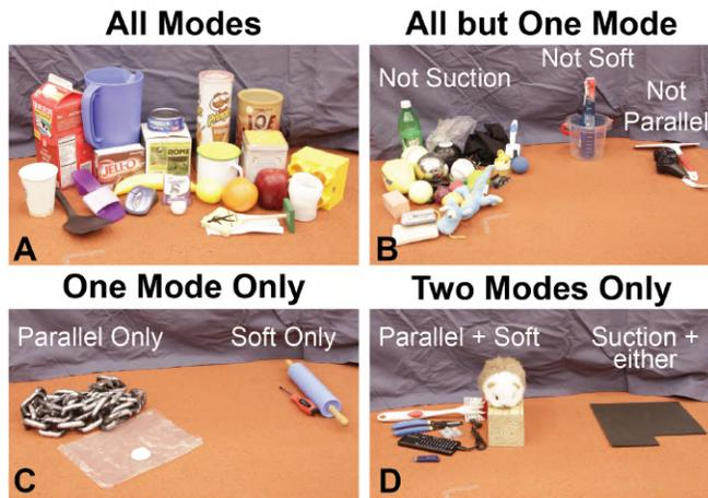
Fig. 5. Subdivision of all graspable objects by which modalities could grasp them. (A) Objects that could be grasped by all modes. These tended to be larger or have one smooth flat surface. (B) Objects that could be grasped by all but one mode. Suction notably had significant difficulty with curved objects and rough surfaces. (C) Objects that could be grasped by only one mode. (D) Objects that could only be grabbed by a combination of grasping modes.
