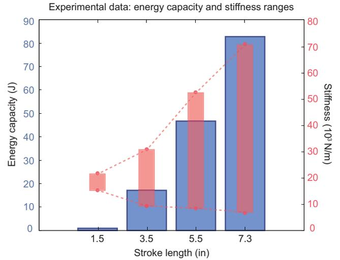
Fig. 4. Experimental results of the range of stiffness and the energy storage capacity of the air cylinder, for different equilibrium height,  $z_0$ , and stroke length. The maximum energy storage capacity and the stiffness modulation range both increased as more air was added into the cylinder.
