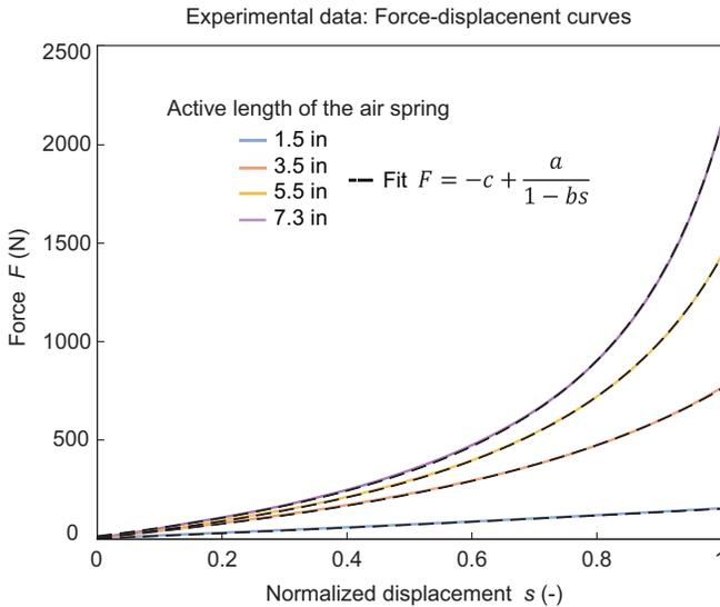
Fig. 3. Experimental result of the spring force (N) versus the normalized deformation of the spring  $s = (z - z_{\min}) / (z_0 - z_{\min})$ . Four compression trials were performed with cylinder stroke lengths of 1.5, 3.5, 5.5, and 7.3 inches measured from the same lowest compression height  $z_{\min}$ . The deformation was normalized with the corresponding  $z_0 - z_{\min}$  value for each trial.
