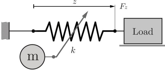
Fig. 1. Model of a variable stiffness spring. In this model,  $z$  denotes the length of the spring,  $F_z$  denotes the force by the spring, while  $k$  denotes the stiffness of the spring changed by the “motor”  $m$ .
