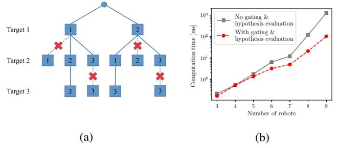
Fig. 2: (a): Hypothesis tree for three targets and three measurements after gating.  $\emptyset$  is omitted for simplicity. The set of valid hypotheses is  $\{(1, 2, 3), (2, 1, 3)\}$
