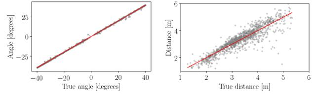
Fig. 3: Vision-based measurement models: (a) bearing; (b) distance. Red line: model v.s. true value, gray dots: measurement v.s. true value.
