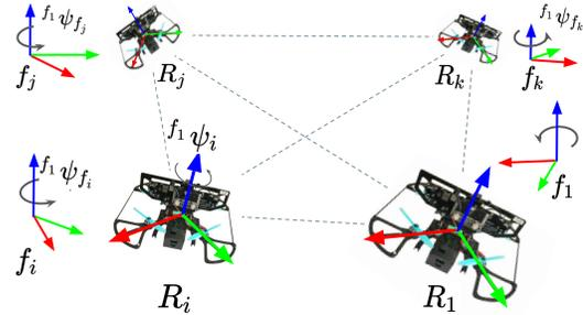
Fig. 1: An example of a homogeneous 4-MAV system featuring our Falcon 250 platform [22]. Robot  $i^{th}$  is associated with a body frame  $i$  and a fixed frame  $f_i$ .  $f_1$  is chosen to be the common fixed frame. Each robot can detect other robots but not their identity. There are errors in detection and tracking. The robots can communicate with each other.
