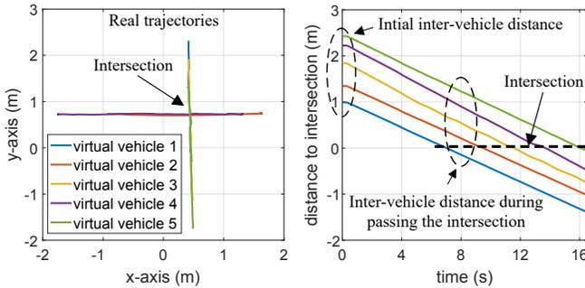
Fig. 7. Results of the non-stop intersection passing experiment.
