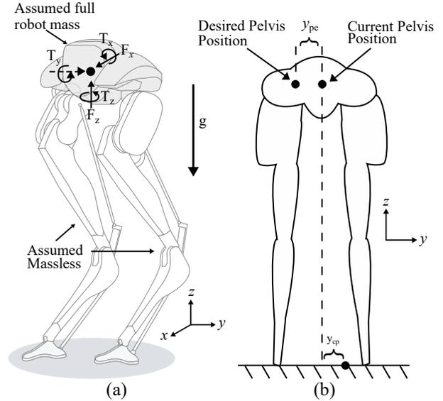
Fig. 3. (a) Cassie is controlled by commanding the listed forces and torques on the pelvis. The pelvis is assumed to be the only component with mass. (b) Cassie can regulate its  $y$  position of its pelvis by controlling the desired center of pressure.
