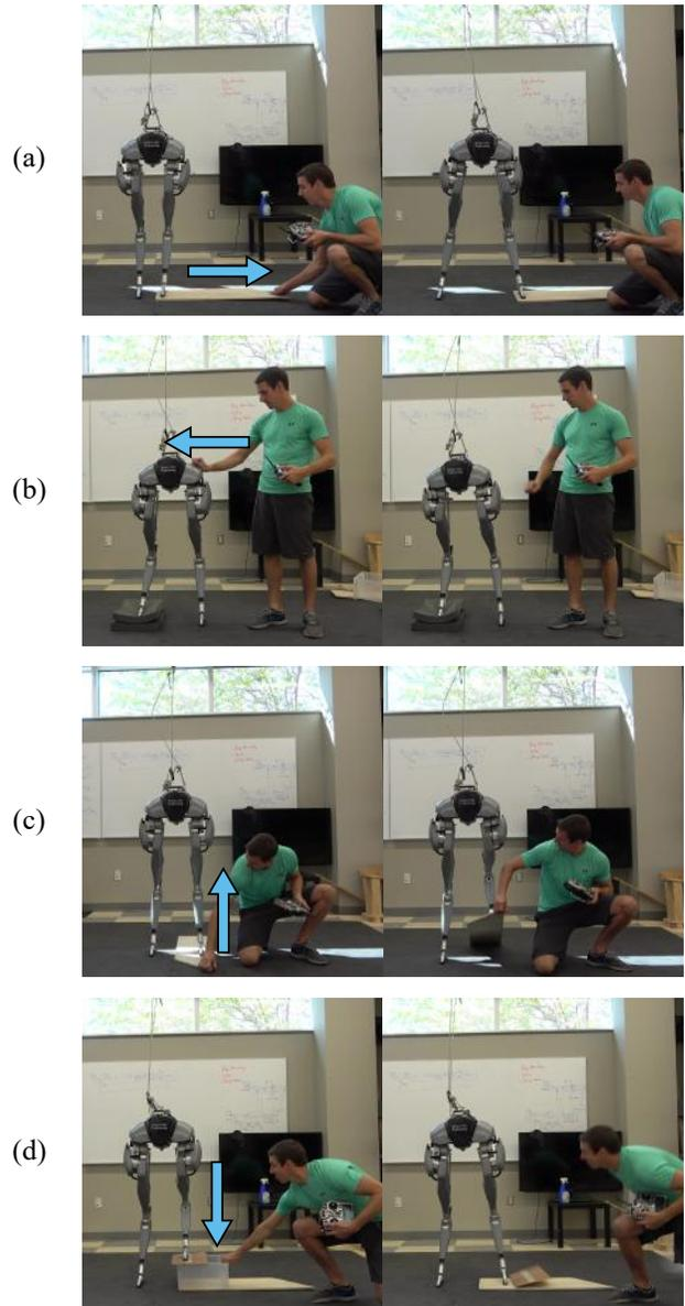
Fig. 6. Examples of different perturbations applied on Tallahassee Cassie. (a) “Leg Spread”: Cassie’s foot is moved by sliding a board. (b) “Soft Foam and Push”: One of Cassie’s feet is supported by soft foam and the pelvis is pushed. (c) “Lift and Lower”: Cassie’s foot is raised and lowered using a board. (d) “Box Drop”: A box is quickly pulled from under Cassie’s foot, forcing it to recover from a fall.
