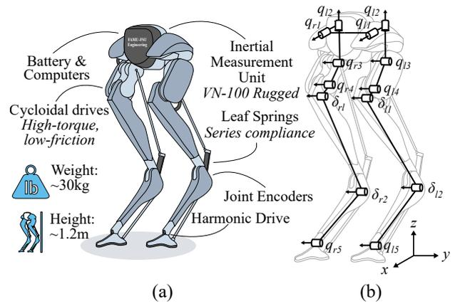
Fig. 4. (a) Overview of Cassie's hardware and basic features. (b) Kinematic diagram of Cassie showing motor positions and spring deflections.
