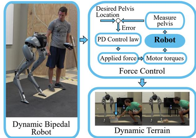
Fig. 1. We implement a force-based controller for balancing the bipedal robot, “Tallahassee Cassie” on dynamic terrain, such as soft terrain or a sudden loss of foot contact.
