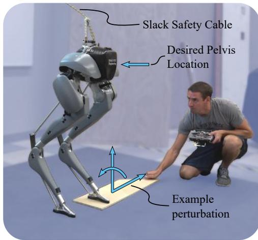
Fig. 5. Experimental setup for testing the balancing controller on Tallahassee Cassie for each of four balance perturbations.
