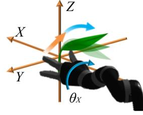
Fig. 3. A schematic of the coordinate system. The pulling and rotation of plucking are described by the  $Y$ ,  $Z$ ,  $\theta_x$  displacements.
