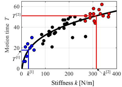
Fig. 5. Relation between stiffness  $k$  and motion time  $T$  in the taught data. The time length of a new motion is determined based on the relation.
