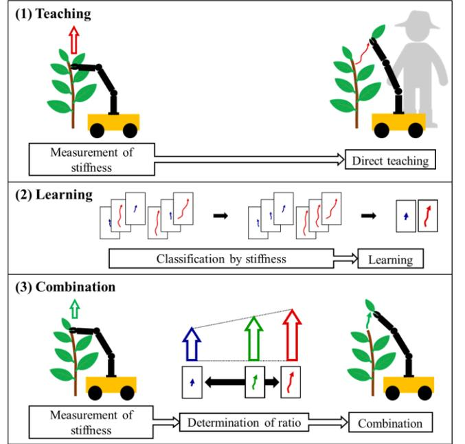
Fig. 4. Proposed system flow. The robot measured the stiffness of the branches, to judge the condition which affected the plucking motion.
