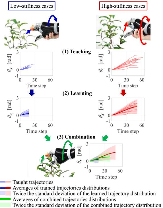
Fig. 2. Outline of proposed system. The proposed system has three steps. First, humans directly teach the robot the plucking motions for small and large values of branch stiffness. Second, the taught motions are learned for each case. Third, the motion that interpolates the two learned motions is generated by probabilistically combining them.
