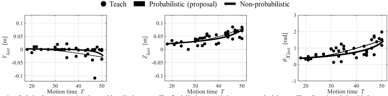
Fig. 6. Relation between motion time and last displacement. The final displacement is important to pluck leaves. Therefore, the relationship between the motion time and last displacement was compared.
