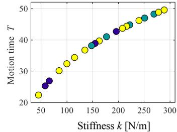
Fig. 9. Relation between stiffness  $k$  and results. When the measured stiffness was intermediate, an intermediate plucking motion was generated to pluck the leaf corresponding to the measured stiffness.
