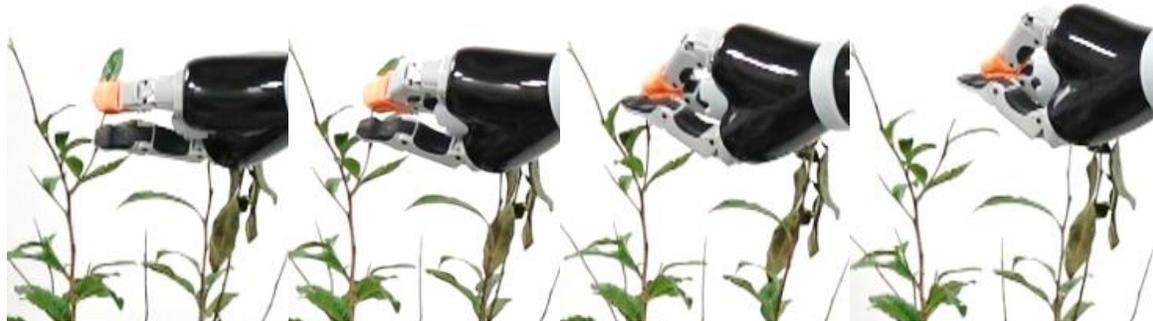
Fig. 11. Plucking motion generated by the proposed method. The complex plucking motion, with pulling and rotation, was reproduced.
