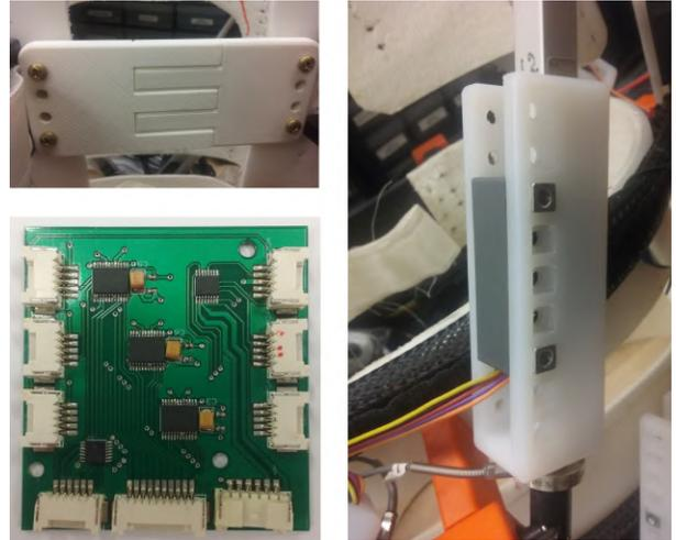
Fig. 2. Upper Left: ring spacer; Lower Left: motor driver and multiplexer PCB; Right: motor housing.
