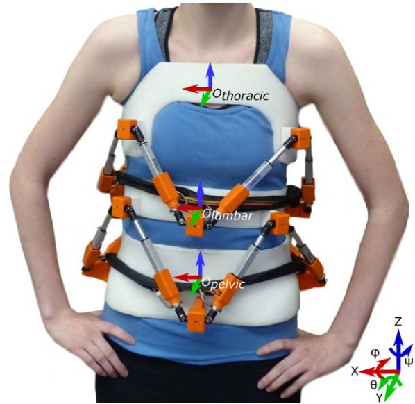
Fig. 1. Robotic Spine Exoskeleton designed for adolescent females
