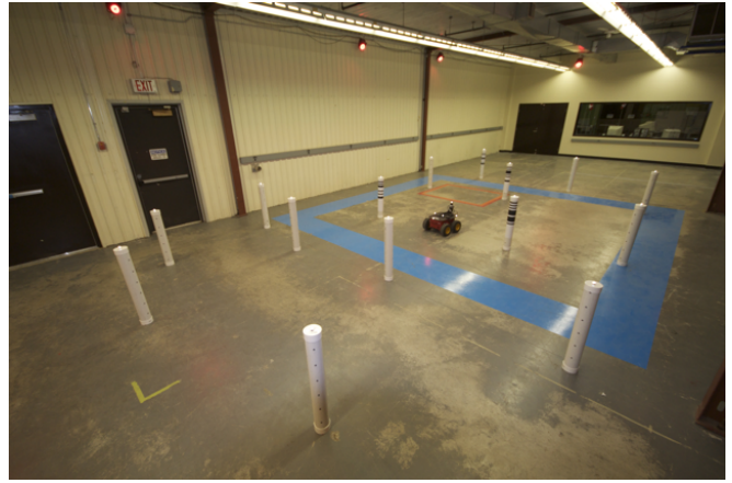
Fig. 6. Experimental setup of the ‘Lost in the Woods’ dataset, courtesy of [Barfoot2009]. Truth measurements are obtained from a motion capture system.
