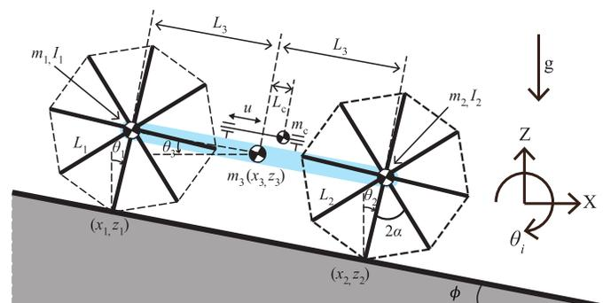
Fig. 1: Combined rimless wheels with active wobbling mass
