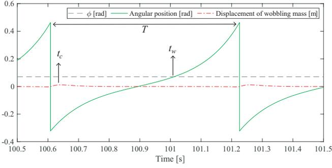
Fig. 5: Normalized phase difference between walker and wobbling mass in entrained limit cycle
