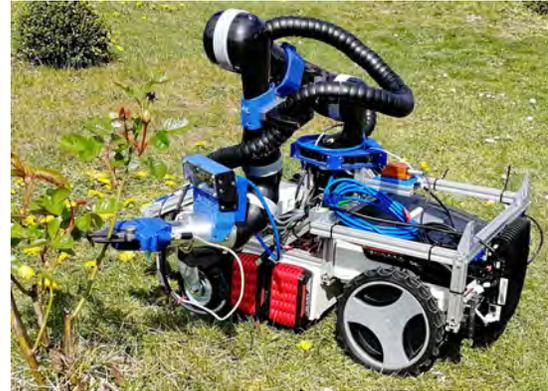
Fig. 1: Overview photo of the rose cutter robot.
