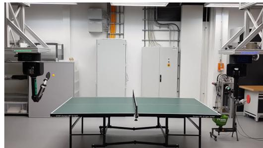
Fig. 1: Robot table tennis setup used to evaluate the trajectory forecasting methods. The ball is tracked using four VGA resolution cameras attached to the ceiling with a sampling frequency of 180 frames per second. The robot arms are Barrett WAM capable of high speed motion with seven degrees of freedom.
