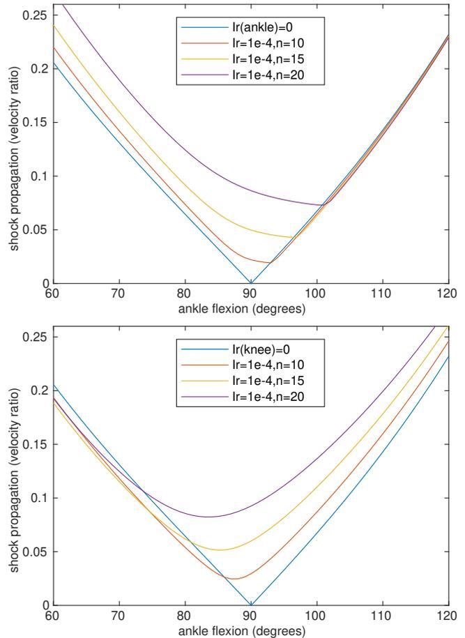
Fig. 5. Plots of shock propagation versus ankle angle for various values of ankle (top graph) and knee (bottom graph) rotor inertia and gear ratio, for the same leg design as in Figure 3 ( $r_2 = 0.2\text{m}$ )
