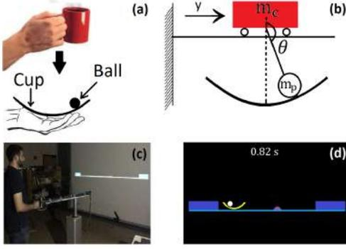
Fig. 1. (a) Real and simplified task. (b) Mechanical model. (c) Virtual environment with a subject operating the HapticMaster robot to manipulate the virtual cup. (d) Screen display.
