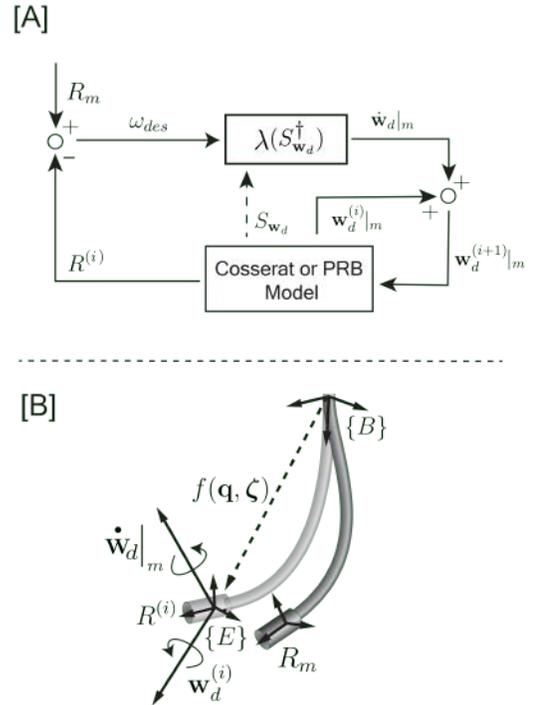
Fig. 1. Iterative disturbance estimation algorithm. [A] Block diagram illustrating the iterative update of the disturbance based on inclinometer data. The initial value for  $\mathbf{w}_d^{(i)}$  is obtained after initial calibration. [B] The compliance matrix  $S_{w_d}$  is used to minimize the orientation error between current estimated orientation  $R^{(i)}$  and the measured value from the sensors  $R_m$ .
