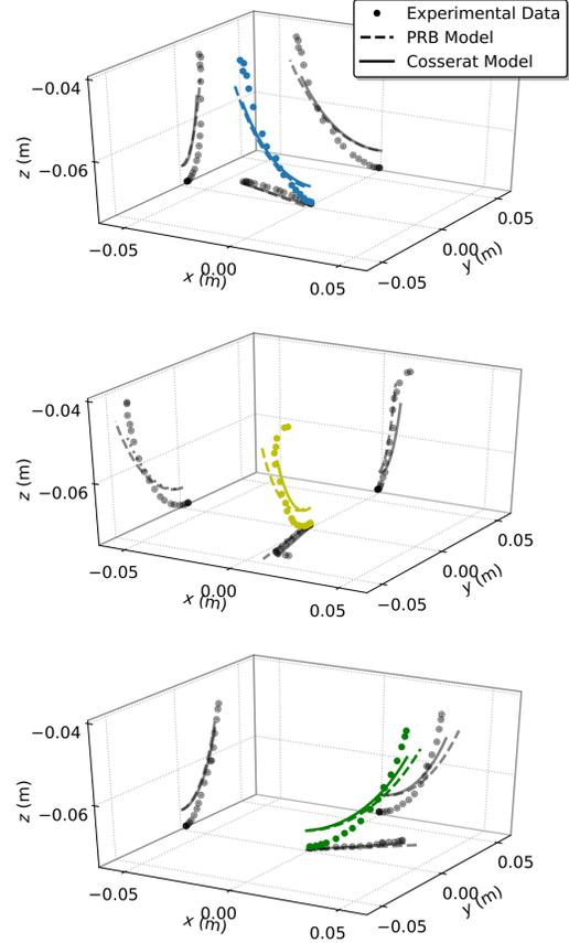
Fig. 4. Experimental validation of the calibrated coefficient  $\zeta^*$ . Each sweep is marked with a different color. The experimental deflection (dots) is projected on  $xy$ ,  $xz$ ,  $yz$  planes together with the corresponding position estimated from both PRB (black dashed line) and Cosserat (black continuous line) frameworks.
