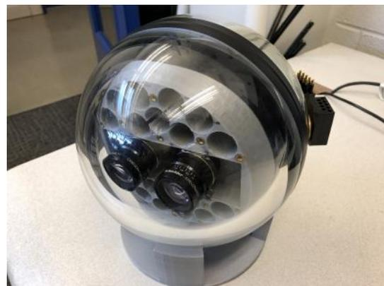
Fig. 1: Stereo camera used for vehicle navigation. The position of the cameras is far from the center of the hemisphere, introducing significant distortion in the images.
