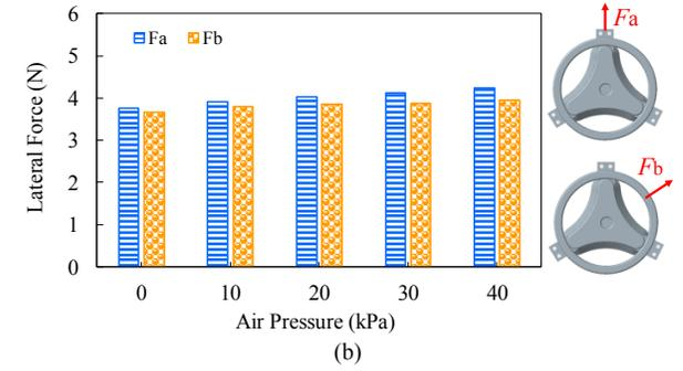
Figure 5. Lateral stiffness tests. (a)  $\Delta L = 0$  mm;  $D = 2$  mm;  $P_1 = P_2 = 40$  kPa;  $P_3 = 0, 10, 20, 30, 40$  kPa. (b)  $\Delta L = 0$  mm;  $D = 2$  mm;  $P_1 = P_2 = P_3 = 0, 10, 20, 30, 40$  kPa.
