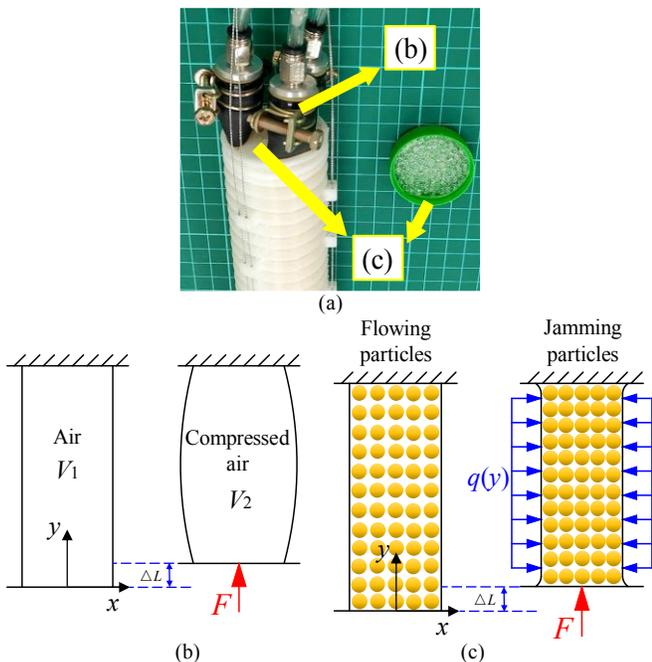
Figure 2. Working principle of the particle jamming pressure change. (a) Diagram of the air and particle chambers. (b) Air chamber compression. (c) Particle chamber compressed by tendon pulling force  $F$  and air pressure from three chambers.
