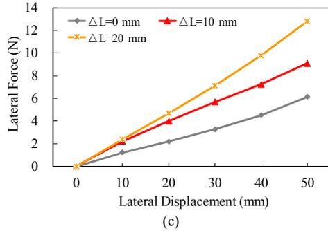
Figure 4. Lateral stiffness tests. (a)  $\Delta L = 0$  mm;  $D = 2$  mm;  $P = 0, 10, 20, 30, 40$  kPa. (b)  $\Delta L = 0$  mm;  $D = 1, 2, 3$  mm;  $P = 0, 10, 20, 30, 40$  kPa. (c)  $\Delta L = 0, 10, 20$  mm;  $D = 2$  mm;  $P = 20$  kPa.
