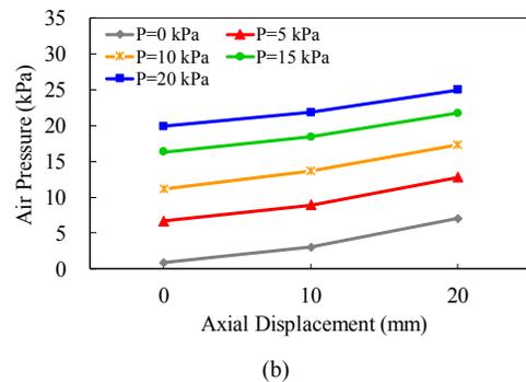
Figure 7. Air pressure changes at different axial displacements and initial pre-charged air pressures. (a) Air pressure test platform. (b) Air pressure test results.
