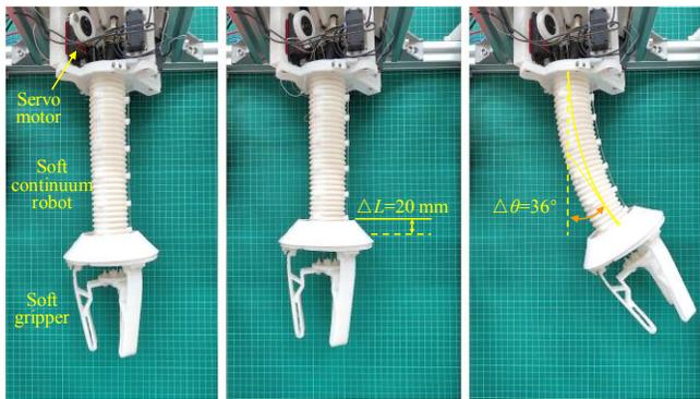
Figure 8. Soft continuum robot moving range.
