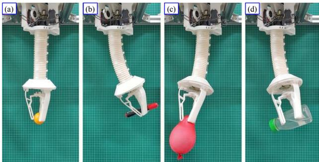
Figure 9. Demonstration of sample grasping. (a) Table tennis ball (2.85 g). (b) Pen (16.76 g). (c) Balloon (1.06 g). (d) Water-filled bottle (162.45 g).
