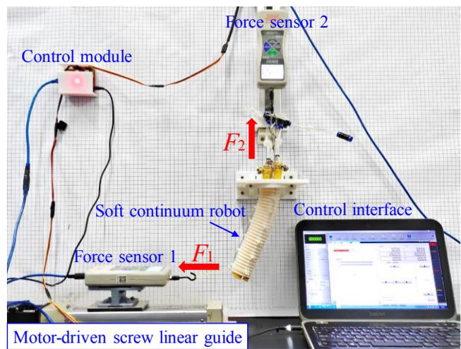
Figure 3. Stiffness test platform.
