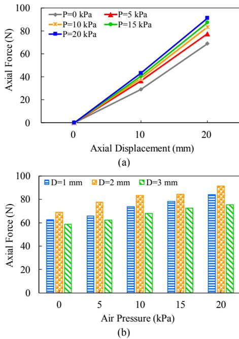
Figure 6. Axial stiffness tests. (a)  $\Delta L = 0, 10, 20$  mm;  $D = 2$  mm;  $P = 0, 5, 10, 15, 20$  kPa. (b)  $\Delta L = 20$  mm;  $D = 1, 2, 3$  mm;  $P = 0, 5, 10, 15, 20$  kPa.
