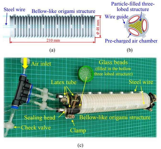
Figure 1. Basic design concept. (a) The bellow-like origami structure. (b) A cross-section showing the three-lobed structure filled with particles and three air chambers. (c) A prototype.
