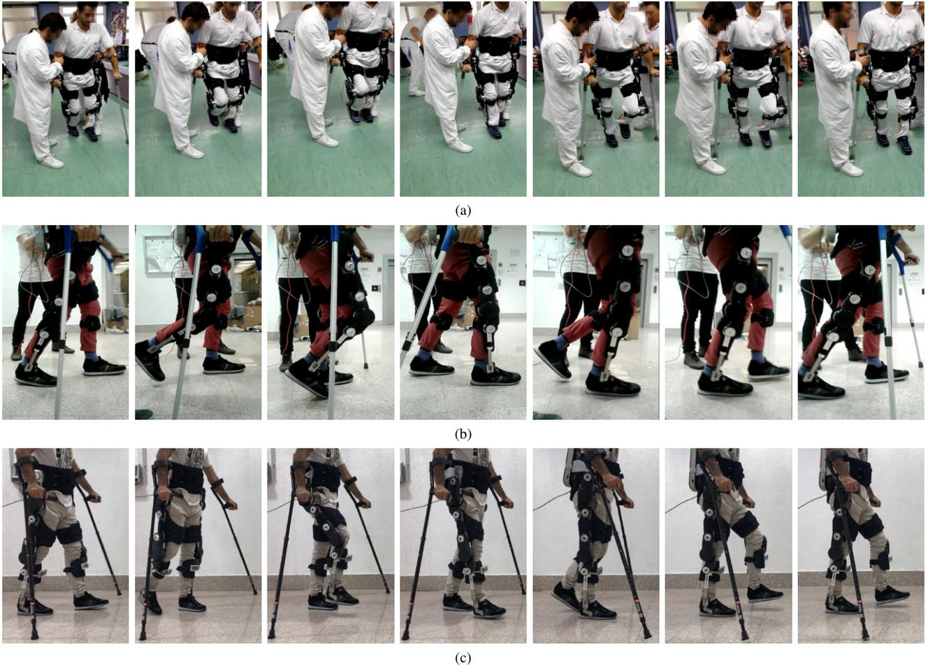
Fig. 7: Snapshots of the experiments (a) SCI patient testing the T1 trajectory at the Centro Protesi INAIL premises. (b) Healthy subject stumbling on the ground while testing the T2 trajectory at the Rehab Technologies Lab premises. (c) Healthy subject testing the T3 trajectory at the Rehab Technologies Lab premises.
