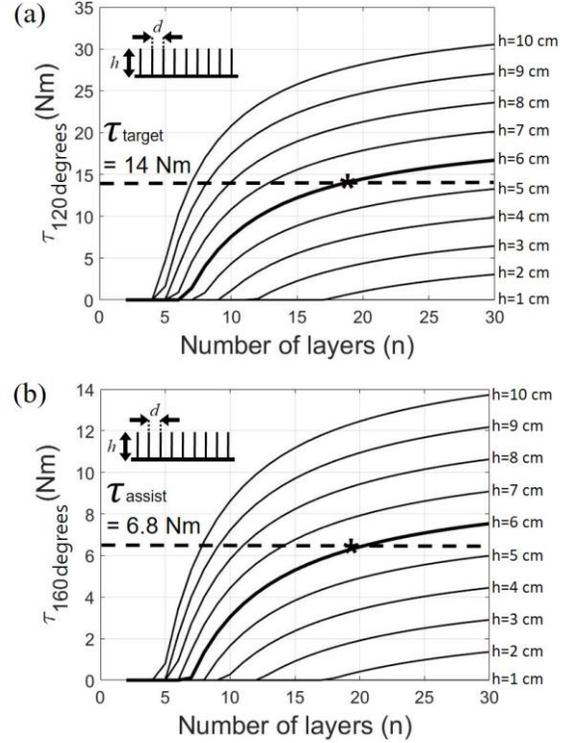
Fig. 5. (a) Torque at 120° estimated from the theoretical model for different numbers of layers ( $n$ ) and heights of the layer ( $h$ ). The black dotted line indicates the target torque generated by the inflatable actuator. (b) Torque at 160° estimated from the theoretical model for different numbers of layers ( $n$ ) and heights of the layer ( $h$ ). The black dotted line indicates the torque generated by the inflatable actuator.
