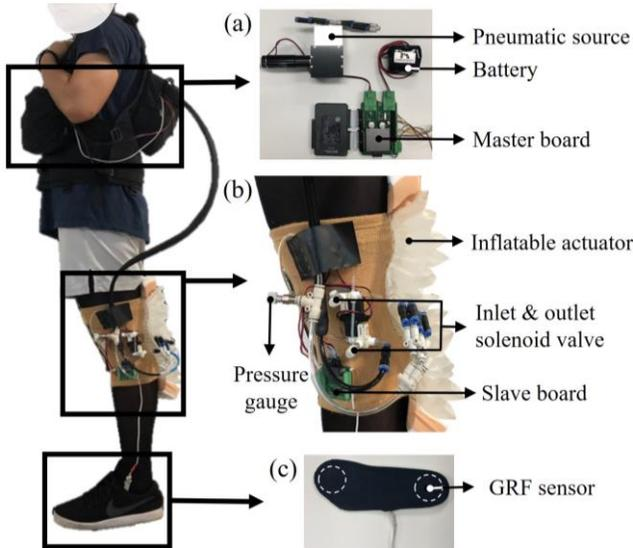
Fig. 9. Developed wearable knee suit. (a) Controller and pneumatic source inside the bag: air is supplied by the portable pneumatic power source, which is controlled by the master board. (b) Knee exosuit: air is controlled by the solenoid valves, and the pressure gauge measures the pressure in the actuator. (c) Ground reaction force (GRF) sensors: the user intention is detected by the insole-type GRF sensors embedded in the shoe.
