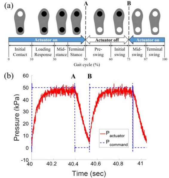
Fig. 10. (a) Actuator-on and -off periods according to the operation of the GRF sensors. (b) Pressure at the inlet of the actuator and command pressure generated by the controller according to the user intention during the walking test.
