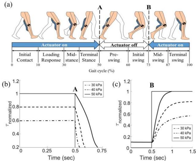
Fig. 8. (a) Actuator on and off periods according to the gait cycle. The actuator is deflated at point A and inflated at point B. (b) Deflation response of the actuator at point A for various pressures on all layers. (c) Inflation response of the actuator at point B to various input pressures on the operated layers, with 50 kPa filled in the non-operated layers.
