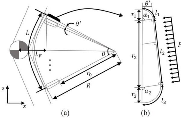
Fig. 4. (a) Geometric representation of the actuator in the inflated state demonstrating interactions among the layers. (b) Cross section of an individual layer showing the dimensions of the theoretical model.
