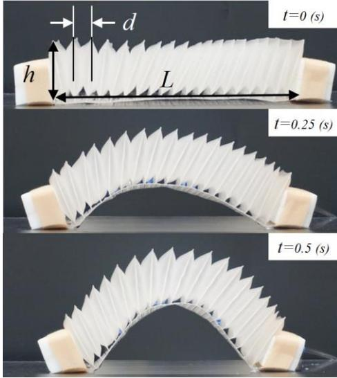
Fig. 2. An inflatable actuator before and after inflation with the dimension descriptions of the height of the layers ( $h$ ), the distance between the layers ( $d$ ), and the length ( $L$ ) of the actuator.
