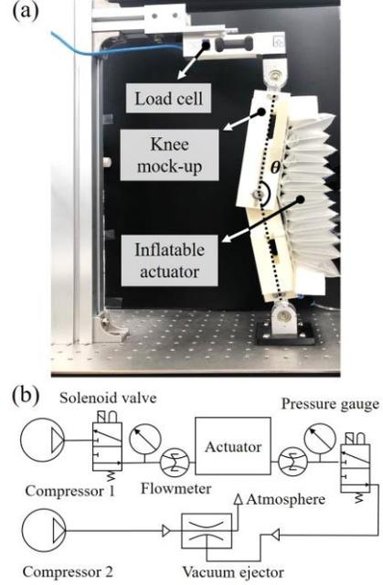
Fig. 6. (a) Experimental setup used to measure the torque generated by the actuator. (b) Pneumatic circuit diagram used to reduce the deflation time by using a vacuum ejector.
