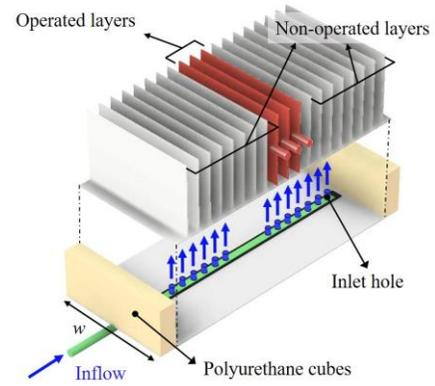
Fig. 3. Graphical illustration of the inflatable actuator: the non-operated layers are inflated through inlet holes connected to one inlet port (see blue arrows). Two polyurethane cubes are attached to both ends of the actuator to support the layers.
