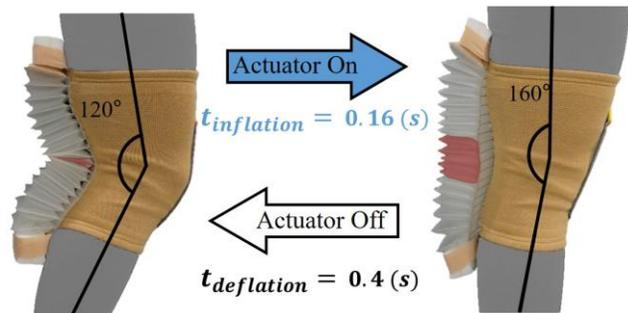
Fig. 1. Wearable knee suit with an inflatable wrinkle actuator to assist knee flexion and with fast inflation/deflation responses obtained via partial control of the wrinkle structure.
