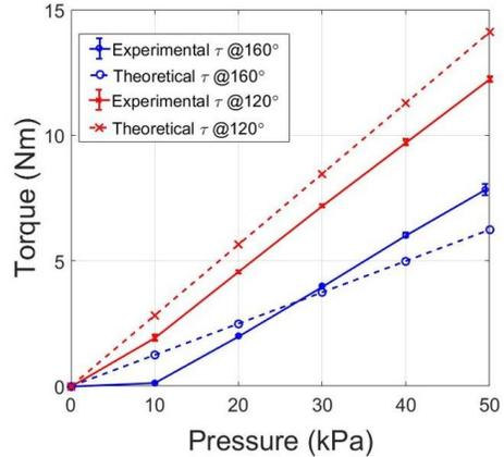
Fig. 7. Theoretically estimated torque versus experimentally measured torque.
