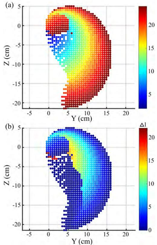
Fig. 5. Reaching a position in different length configurations. (a) Minimum length needed to reach the point lying in  $YZ$  plane and (b) The maximum difference in length which can be used to reach a point in the workspace.
