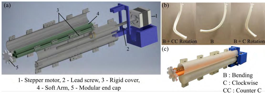
Fig. 2. VaLeNS arm: (a) Different components and their assembly. (b) The different deformation modes of  $BR^2$  SCA (B:Bending, C: Clockwise rotation and CC: Counterclockwise rotation). (c) Fabricated prototype of the VaLeNS arm used in this work.
