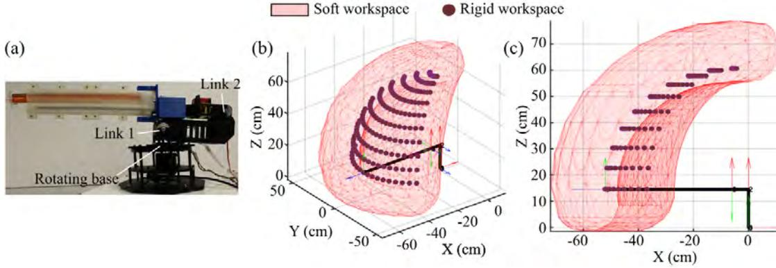
Fig. 6. (a) VaLeNS arm attached to a 3-link robotic arm and its adaptable and precise workspace obtained ((b)isometric view and (c) XZ view) with the ranges of 3 link robotic arm limited to  $-45$  to  $45$  deg. for the rotating base, Link 1 fixed at  $90$  deg. and Link 2 varied from  $0$  deg. to  $90$  deg.
