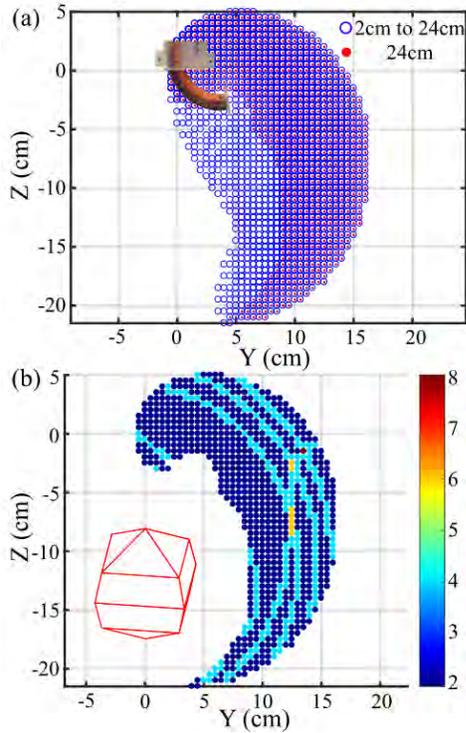
Fig. 4. (a) Workspace of the VaLeNS arm with its entire length extruded (24 cm) and varying extruded lengths (from 2 cm to 24 cm) and (b) Dexterity of the  $BR^2$  SCA with its service sphere shown in the inset. For example, a workspace point with cyan color can be reached in four unique orientations (the center of the service sphere [23] is reached such that the tangents pass through four different faces of the service sphere)
