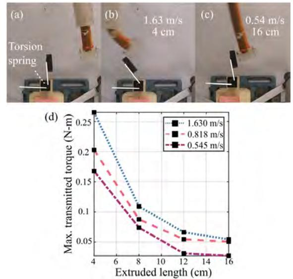
Fig. 7. (a) Impact test setup where a torsion spring is fixed, the maximum deflection of the torsion spring obtained when impacted with the VaLeNS arm extruded to lengths of (b)  $4$  cm and tangential velocity  $1.63$  m/s, (c)  $16$  cm and tangential velocity  $0.54$  m/s and (d) maximum transmitted torque when impacted with different SCA extruded lengths and tangential velocities.
