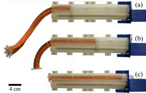
Fig. 1. The Variable Length Nested Soft arm or VaLeNS arm with (a) the soft arm completely extruded, (b) partially extruded, and (c) completely retracted within a rigid shell.
