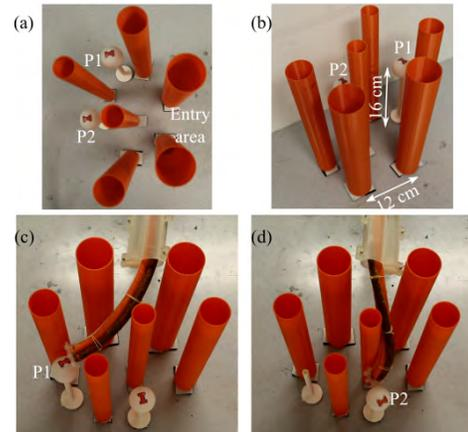
Fig. 9. (a)-(b) Obstacle course for the reachability tests showing the entry area and locations of the objects(P1,P2) to be reached.(c)-(d) final poses of the VaLeNS arm reaching P1 and P2 respectively.
