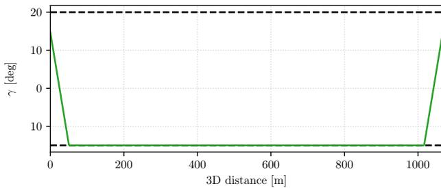
Fig. 3. Example of the computed 3D path by the proposed heuristic approach for the instance Long 3. The minimum turning radius  $\rho_{\min} = 40$  m and the limit for the pitch angle  $\Gamma = [-15^\circ, 20^\circ]$ . The results are supplemented with computed curvature and altitude profiles.
