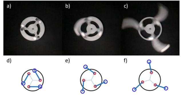
Figure 9. Spoke-open in high speed rotation. a)-c) are spoke-open is real. d)-f) are simulated figure. by a),d) zero-speed, b),e) Spoke spread-speed ( $\omega_{spread} = 52.16 \text{ rad/s}$ ), and c),f) high-speed.
