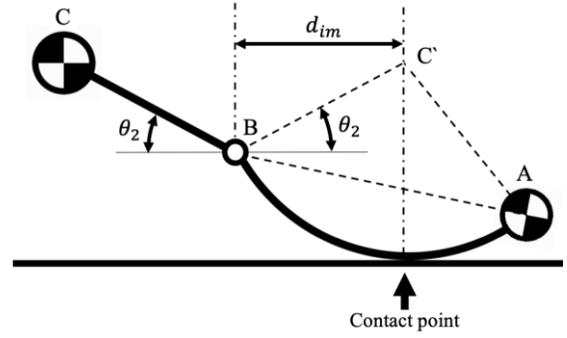
Figure 6. Free-body diagram of the spoke in the impact case.  $d_{im}$  is the horizontal distance between the contact point and joint B, and it can be derived by the geometrical shape. The impact force acts on the spoke at the contact point. Note that line  $BC$  and line  $BC'$  have the same length as  $l_2$ .
