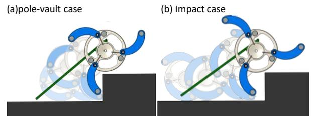
Figure 3. The scenarios of the proposed shape-morphing wheel for traversing obstacles. (a) pole-vault case, and (b) impact case.
