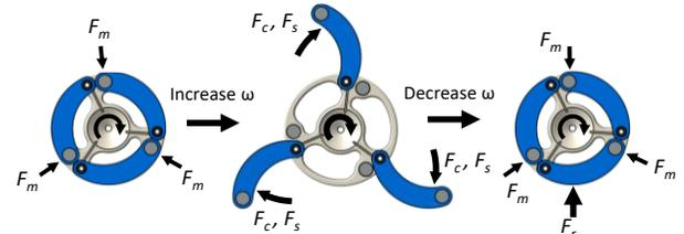
Figure 2. Explanation of the self-morphing function of the wheels according to the operation speed.  $F_m$  is the magnetic force,  $F_c$  is the centrifugal force,  $F_s$  is the spring force, and  $F_r$  is the reaction force from the ground.
