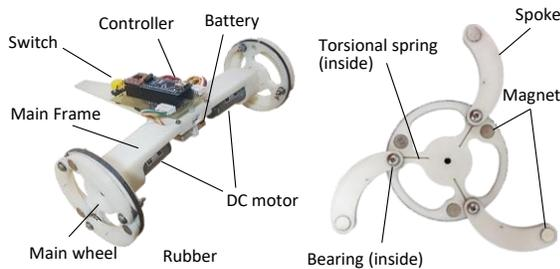
Figure 8. Self-morphing robot prototype for obstacle-overcoming in high speed.
