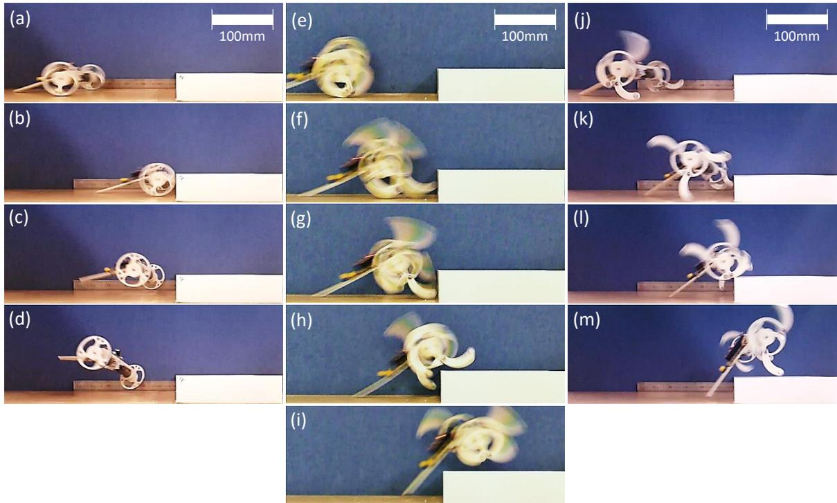
Figure 10. Snapshots during obstacle-traversing. (a)-(d) with static wheels. (e)-(i) pole-vault case, and (j)-(m) impact case (see Multimedia extension).
