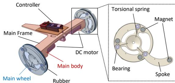
Figure 1. Shape-morphing robot configuration
