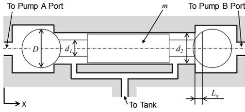
Figure 2. Model of passive flow compensation valve
