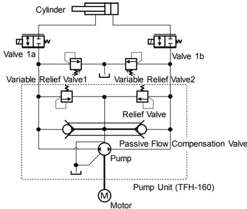
Figure 1. Hydraulic direct-drive circuit
