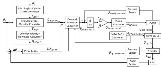
Figure 4. Block diagram of pressure-based control mode
