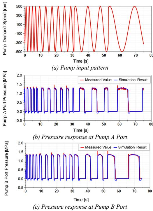
Figure 7. Result of passive flow compensation valve simulation
