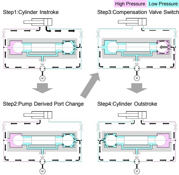
Figure 3. State of the passive flow compensation valve
