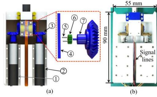
Fig.5 Actuation package of the manipulator, showing (a) the configuration of the actuation package: ① DC-servomotor 1, ② DC-servomotor 2, ③ bevel gear 1, ④ rack, ⑤ pin, ⑥ spur gear, ⑦ bevel gear 2, (b) the photo of the actuation package.
