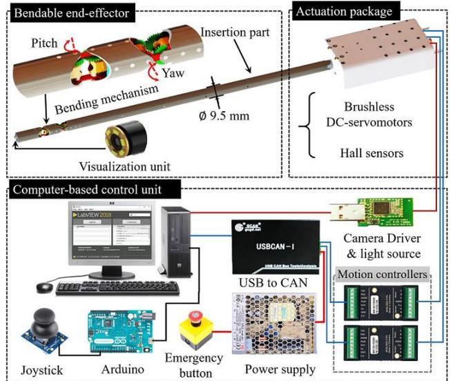
Fig.2 The system configuration of visible manipulator consists of a bendable end-effector with multi-gear array mechanism and visualization unit, an actuation package with brushless DC-servomotors and Hall sensors, and a computer-based control unit.
