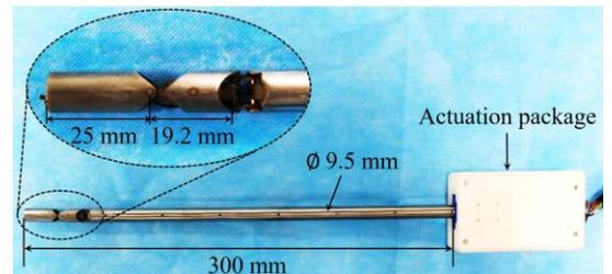
Fig.8 Visible manipulator prototype.
