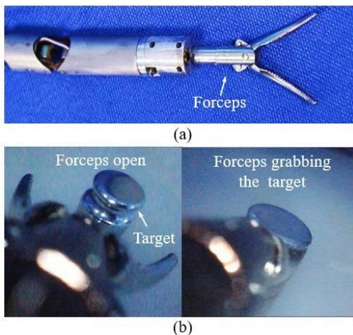
Fig.12 Functional evaluation of visualization unit, showing (a) the forces combined with the visible manipulator, (b) the target and forceps remain within the FOV of the captured endoscopic images.
