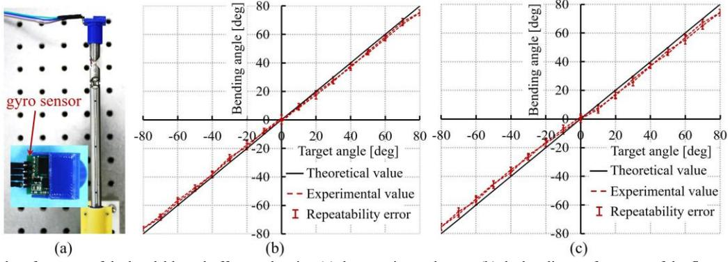
Fig.9 Mechanical performance of the bendable end-effector, showing (a) the experimental setup, (b) the bending performance of the first articulated section, (c) the bending performance of the second articulated section.
