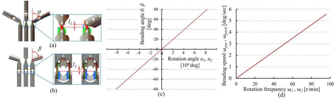
Fig.6 Kinematics analysis of the bendable end-effector, showing (a) the design parameters of the first articulated section, (b) the design parameters of the second articulated section, (c) the kinematic relationship between the bending angle and motor rotation angle, and (d) the kinematic relationship between bending speed and the rotation frequency of the motor.
