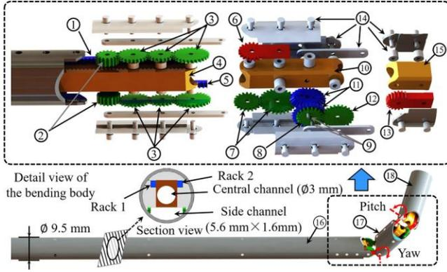
Fig.3 Configuration and detailed view of the bendable end-effector: ① rack 1, ② spur gears 1, ③ gear set 1, ④ base frame 1, ⑤ rack 2, ⑥ shaped gear 1, ⑦ gear set 2, ⑧ spur gears 2, ⑨ pin, ⑩ base frame 2, ⑪ bevel gears, ⑫ spur gear 3, ⑬ shaped gear 2, ⑭ connection frames, ⑮ base frame 3, ⑯ outer frame 1, ⑰ outer frame 2, ⑱ outer frame 3.
