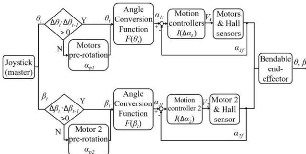
Fig.7 The control strategy for the bending motions.
