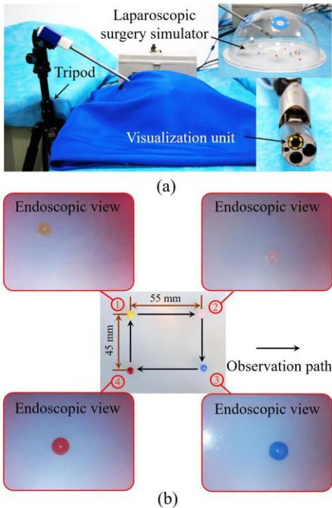
Fig.11 The endoscopic function of the visualization unit, showing (a) the experimental setup, (b) the captured endoscopic images of the target colored beads.
