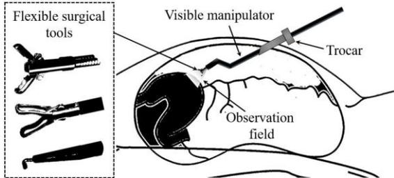
Fig.1 Concept of visible manipulator in laparoscopic surgery.
