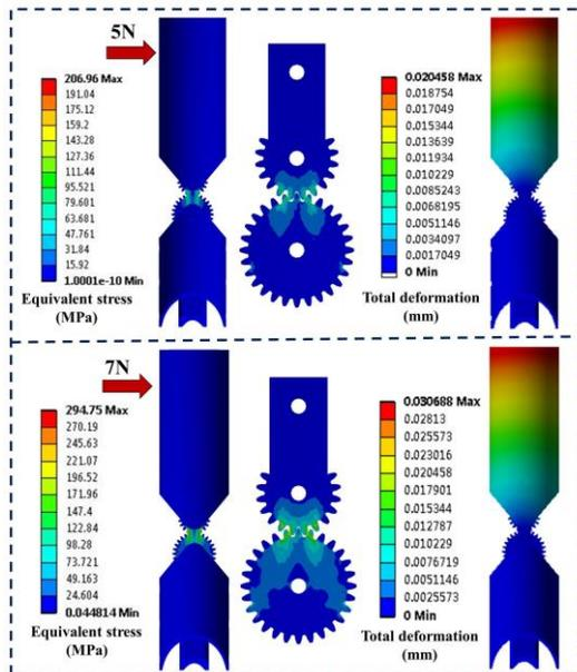
Fig.4 FEA simulation results of the stress and deformation generated in the joint and internal meshing gears under load forces of 5 N and 7 N.
