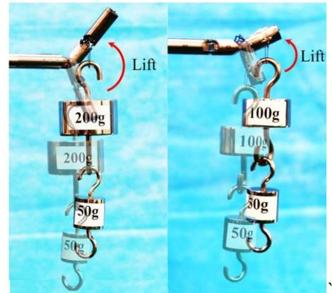
Fig.10 Load capacity of the manipulator.
