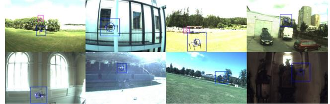
Fig. 1: Examples of annotated footage from the proposed dataset from a disparity of environments. The bounding boxes were generated automatically, using our relative localization system *UVDAR*.
