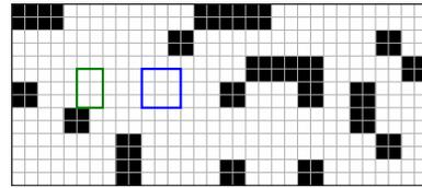
Fig. 1. A  $k = 2$  low-resolution graph with 20% obstacles. The white cells are vertices, and the black cells are obstacles. The green and blue rectangles visualize a  $2 \times 3$  and a  $3 \times 3$  sub-graph.
