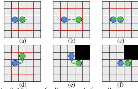
Fig. 3. (a–d) All types of collisions, including collisions on a vertex and head-to-head collisions on an edge, can be contained in some  $3 \times 3$  graphs (drawn in red). (e) The only scenario that we cannot find a  $3 \times 3$  sub-graph due to the black obstacle. (f) We can find a  $3 \times 3$  graph for the scenario in sub-figure (e) by postponing one robot's move.
