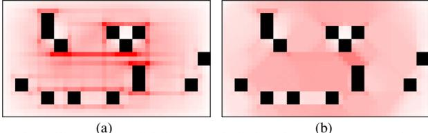
Fig. 6. Comparison of different path finding heuristics in a graph with obstacles visualized in black. Other visual elements are the same as the ones in Fig. 5. (a) Manhattan distance heuristic. (b) Vertex Occupancy heuristic.
