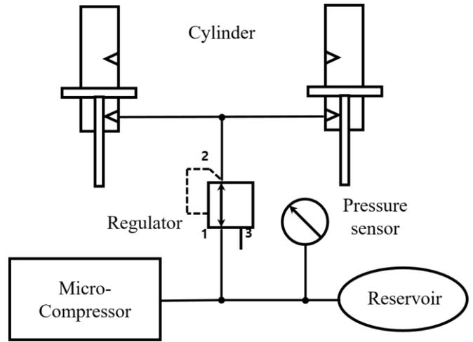
Fig. 5. Pneumatic circuit diagram of proposed system.
