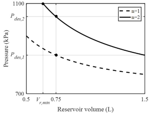
Fig. 8. Desired reservoir pressure ( $P_{des,n}$ ) to volume of reservoir ( $V_r$ ). For example, to actuate the cylinder twice ( $n = 2$ ) with fully charged reservoir, the volume of the reservoir should be at least 0.65 L ( $=V_{r,min}$ ).
