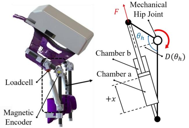
Fig. 2. Mechanical configuration and modeling of developed system.
