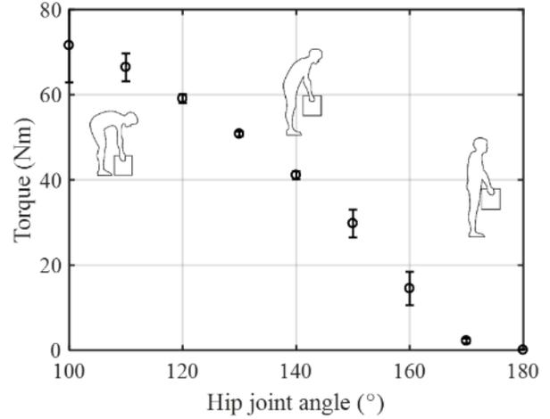
Fig. 4. Ensemble averaged measured output torque with respect to  $\theta_h$  for 6 lifting trials with different lifting speeds. The errorbar represents  $\pm 1$  standard deviation across trials.
