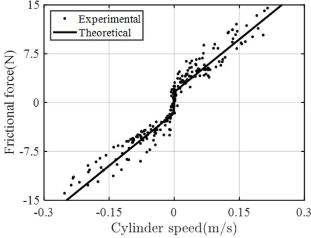
Fig. 3. Model parameters of friction force were identified. The experimental data points are plotted according to cylinder speed ( $\dot{x}$ ) in red dots and the black line is the fitted result ( $\beta = 54.0$ ,  $F_f = 1.62$ ,  $R^2 = 0.953$ ).
