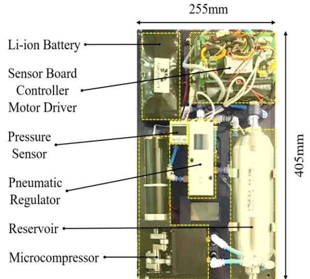
Fig. 6. Components inside the pneumatic actuation pack for generation, accumulation and control of compressed air.
