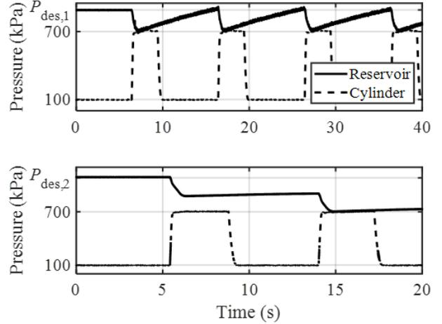
Fig. 10. Reservoir and cylinder pressure under continuous lifting assistance (6 l/m) (a) and assist twice with fully-charged reservoir and without generating compressed air (b).
