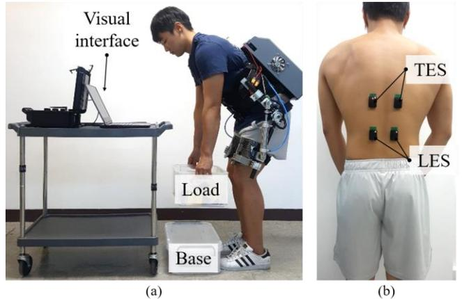
Fig. 11. Experimental setup (a) and sEMG electrode placement for TES and LES muscles (b).
