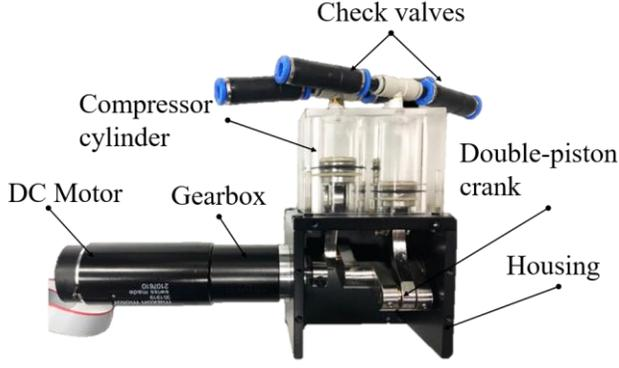
Fig. 9. Structure of customized microcompressor. Ambient air is compressed via double piston crank mechanism.
