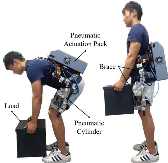
Fig. 1. System overview of a portable pneumatic back support exoskeleton. The system is powered by a pneumatic cylinder and fully portable due to a microcompressor inside a pneumatic actuation pack.
