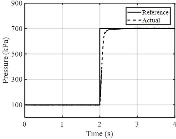
Fig. 7. Reference step input (700 kPa) and actual pressure trajectory. The 10% to 90% rise time is about 100ms.
