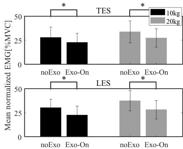
Fig. 13. Mean normalized EMG of TES and LES were reduced with exoskelton compared to noExo conditions.
