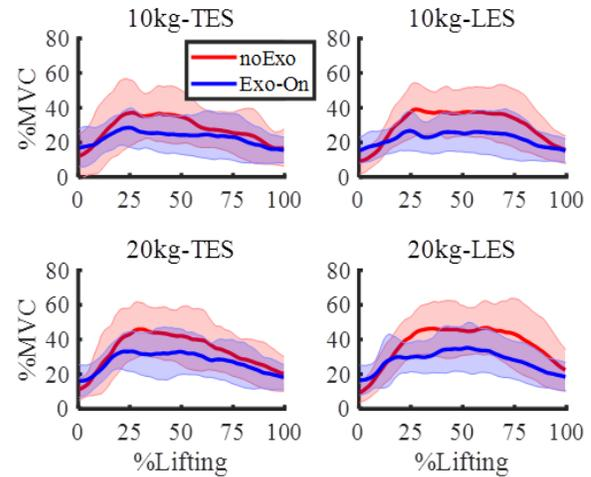
Fig. 12. Muscle activities (%MVC) with respect to lifting cycle (%Lifting) for each muscle (TES/LES) with respect to noExo/Exo and 10 kg /20 kg conditions.
