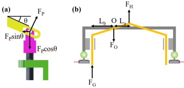
Figure 7 (a) The magnified view of a pin-in-slot joint used between the links. (b) The schematic of the SMP adhesive gripper and the free body diagram of the links.
