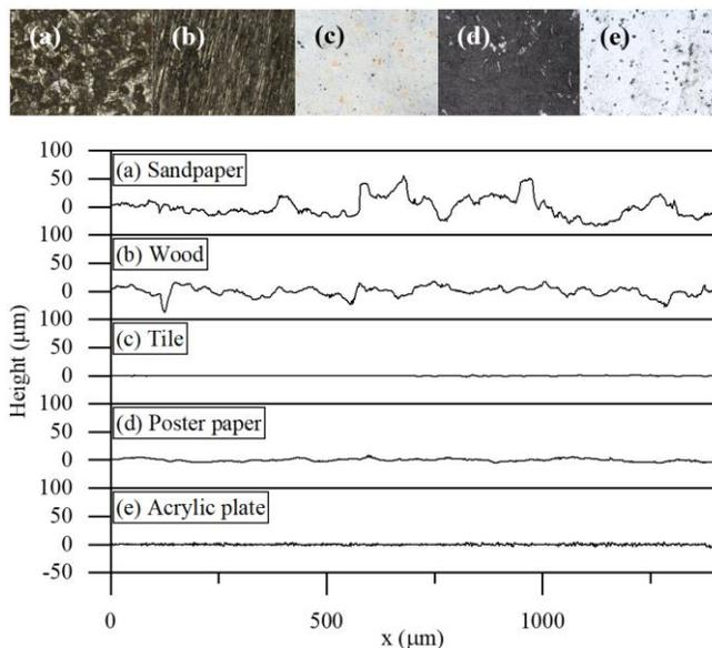
Figure 13 The optical microscope images and the surface roughness profiles of (a) a sandpaper, (b) a wooden plate, (c) a tile, (d) a poster paper, and (e) an acrylic plate used in the picking demonstration in Fig. 12.
