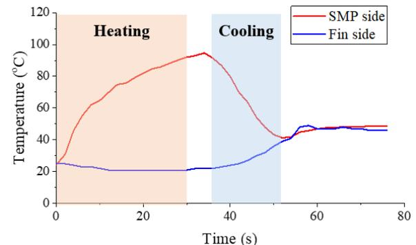
Figure 10 The temperature profile of an SMP adhesive gripper foot during heating and cooling with a Peltier module as a function of time.
