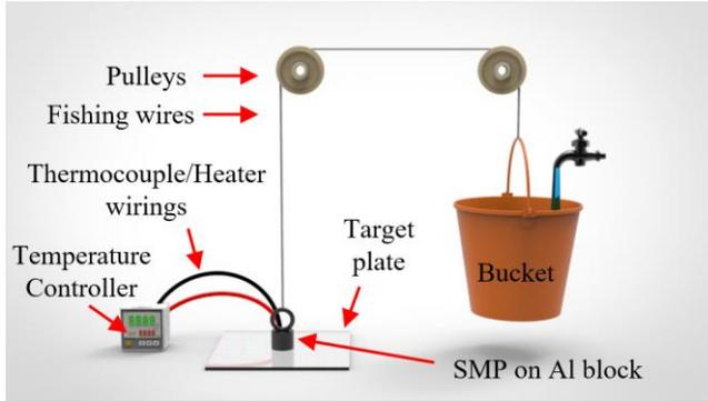
Figure 4 The test setup to measure the adhesion strength of an SMP sample. While an SMP adheres to the target plate, the bucket is filled with water. Once the SMP fails in adhering to the target plate, its adhesion strength is recorded.
