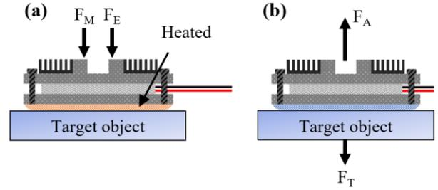
Figure 6 The free body diagram of the foot of an SMP adhesive gripper. (a) Forces during preloading. (b) Forces during picking.
