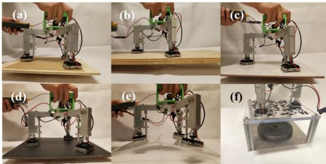
Figure 12 The images of the SMP adhesive gripper picking various surfaces including (a) a sandpaper, (b) a wooden plate, (c) a tile, (d) a poster paper, (e) an angled acrylic plate, and (f) an acrylic plate wet with blue dyed water.
