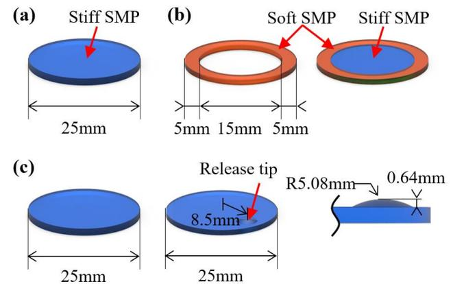
Figure 3 (a) Fabrication of a single SMP sample. A stiff SMP is cured and cut into a 25 mm diameter round shape. (b) Fabrication of a dual SMP sample. A soft SMP is cured and cut into a ring shape and a stiff SMP precursor is subsequently filled and cured inside the ring-shaped soft SMP. (c) Fabrication of an SMP sample with release tip. To form a release tip on a 25 mm diameter SMP sample, a single drop of SMP precursor is placed on the SMP surface and then cured.
