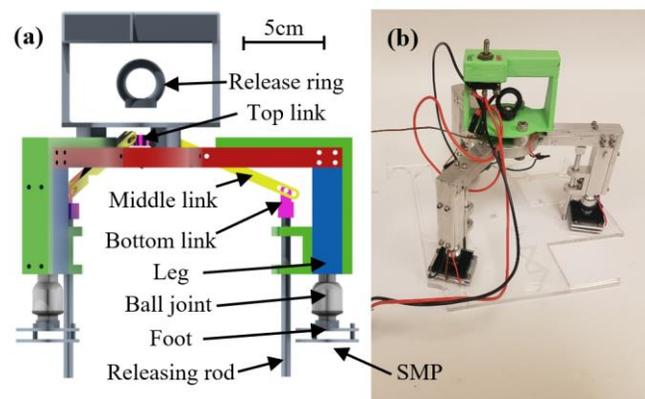
Figure 2 (a) The CAD drawing and (b) the photograph of an SMP adhesive gripper. The gripper has a battery and a thermocouple for heating/cooling and temperature sensing.
