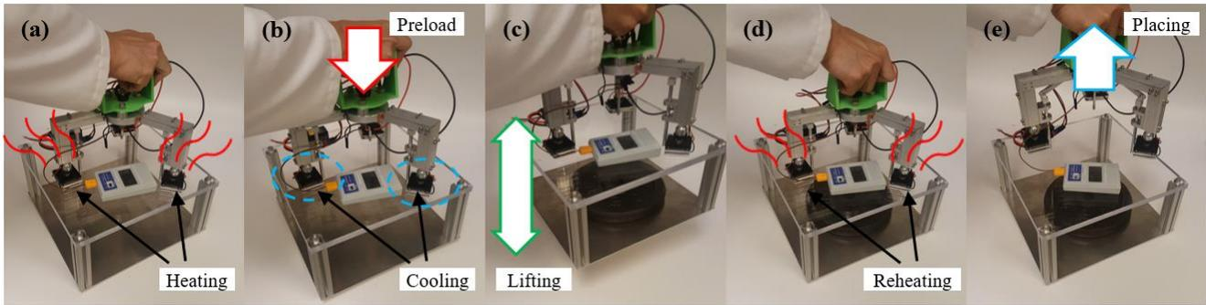
Figure 11 The pick-and-place demonstration of the SMP adhesive gripper.
