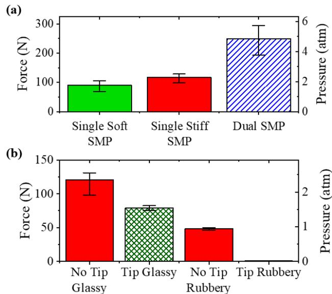
Figure 9 (a) The experimentally measured maximum adhesion strength of single and dual SMPs. (b) The experimentally measured adhesion strength of SMPs with and without release tip in the glassy and rubbery states.
