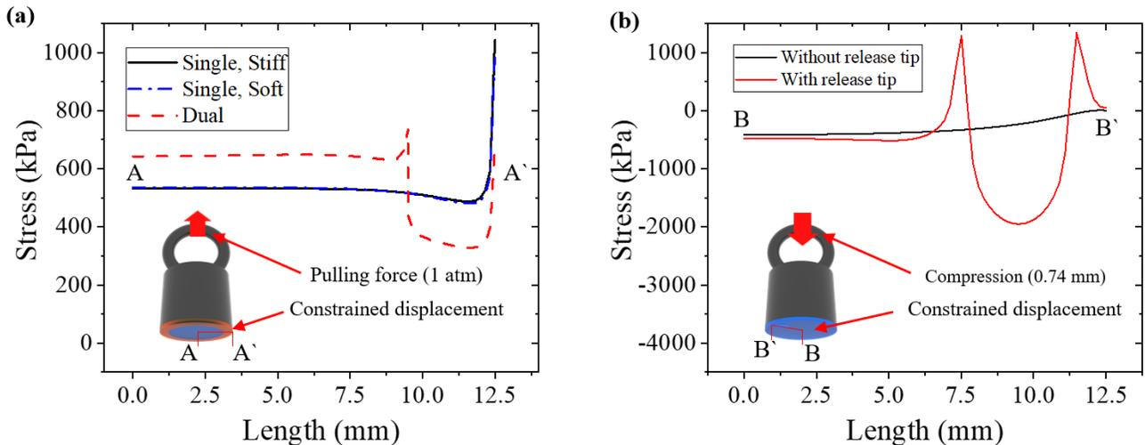
Figure 8 (a) The schematic dual SMP sample attached to the aluminum block with its boundary condition and the plot of the first principal stress along the A-A' line computed using FEA. (b) The schematic SMP with release tip attached to the aluminum block with its boundary condition and the plot of the first principal stress along the B-B' line computed using FEA.
