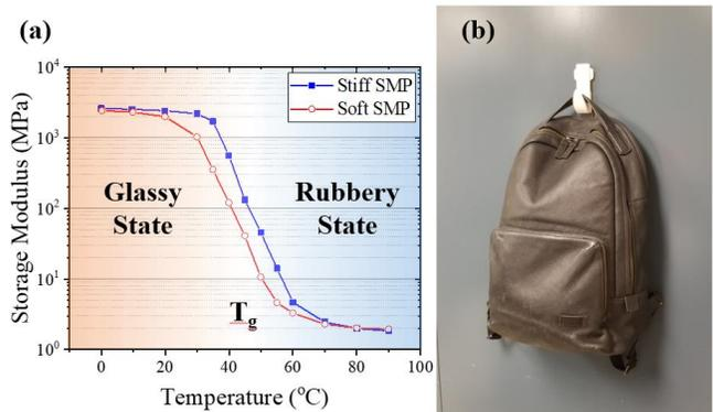
Figure 1 (a) The storage moduli of stiff and soft shape memory polymers (SMPs) as a function of temperature. (b) Application of the SMP for a reversible dry adhesive hook.
