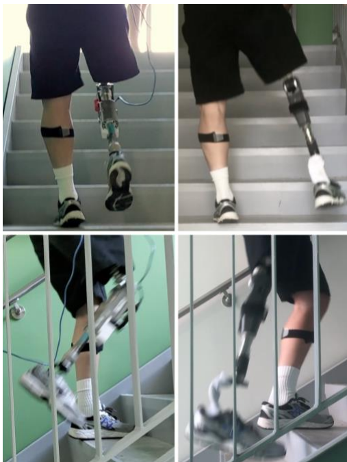
Fig. 7. Subject ascending stairs in a step-over fashion. The left column shows the subject's gait using the SCSA device, the right showing his daily-use device. A video corresponding to these experiments is provided in the supplementary materials.
